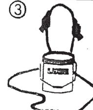
Lubricate the gasket thoroughly before it is placed on the spigot or tongue.
