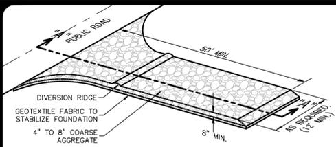
SCHEMATIC OF TEMPORARY CONSTRUCTION ENTRANCE/EXIT
