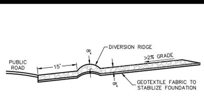
SECTION "A-A" OF A CONSTRUCTION ENTRANCE/EXIT
