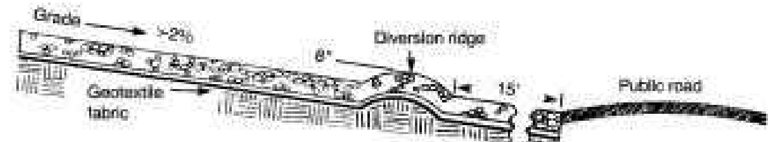
Figure 1-25 Cross-section of a Construction Entrance/Exit (NC, 1993)
