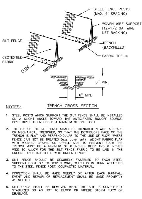
6. ACCUMULATED SILT SHALL BE REMOVED WHEN IT REACHES A DEPTH OF 6 INCHES. THE SILT SHALL BE DISPOSED OF IN AN APPROVED SITE AND IN SUCH A MANNER AS TO NOT CONTRIBUTE TO ADDITIONAL SILTATION. 7. CONTRACTOR SHALL PROVIDE TRIANGULAR SEDIMENT FILTER DIKE
