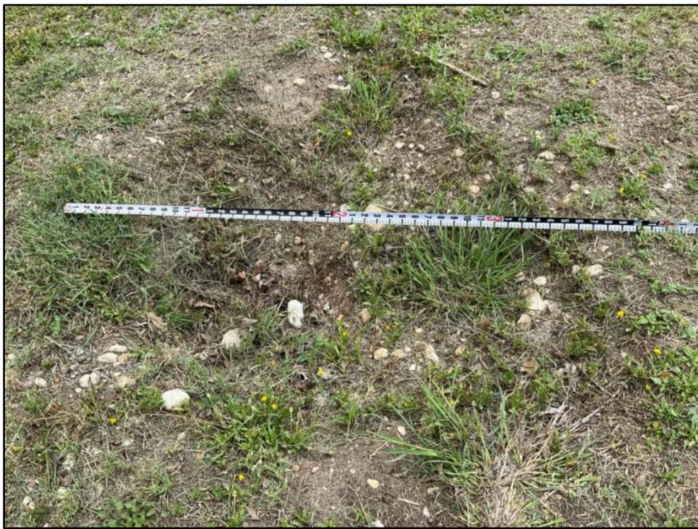
Photo 1. Feature 1. A 3-foot by 3-foot by 10-inch closed depression adjacent to Gruene Road to the west of the Guadalupe River. The depression was filled with organics, fine and coarse soil, and vegetation on initial inspection. Bedrock was not present.
