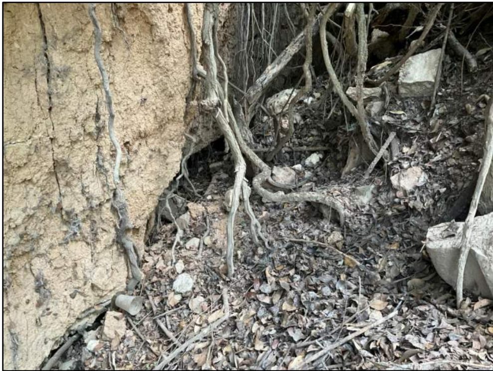
Photo 3. Feature 5. Erosion under clay soil on a hillslope adjacent to Gruene Road to the east of the Guadalupe River. The maximum depth of these voids was 4 feet. Bedrock was not observed. Additionally, this area was located on a topographic high.
