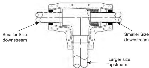
**Continuous Monitoring** - The Dualoy 3000/LCX system has exceptional performance in continuously monitored systems. Due to its small interstitial space, it is very reliable in detecting leaks in systems monitored by pressure, vacuum or hydrostatic methods. False alarms are eliminated by the lesser sensitivity to external conditions while detection capability of actual leaks is increased. Consult NOV Fiber Glass Systems Engineering for details and design of monitoring methods.
