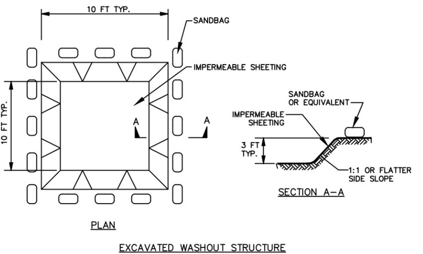
**ONSITE CONCRETE WASHOUT STRUCTURE OR APPROVED EQUAL**
