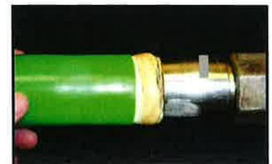
Flexible piping is bulging
