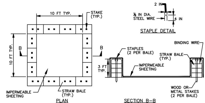
NOTE: CAN BE TWO STACKED BALES OR PARTIALLY EXCAVATED TO REACH 3 FT DEPTH
