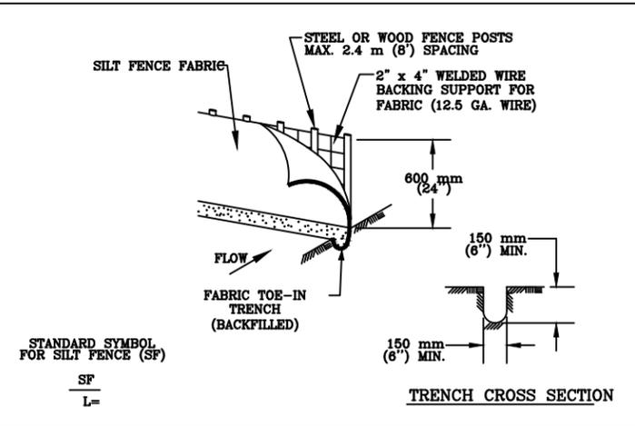
1. STEEL OR WOOD POSTS WHICH SUPPORT THE SILT FENCE SHALL BE INSTALLED ON A SLIGHT ANGLE TOWARD THE ANTICIPATED RUNOFF SOURCE. POST MUST BE EMBEDDED A MINIMUM OF 300 mm (12 INCHES). IF WOOD POSTS CANNOT ACHIEVE 300 mm (12 inches) DEPTH, USE STEEL POSTS.
