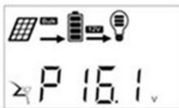
PV panel voltage
