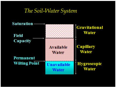
Figure 4.1 The soil-water system showing the various stages of water through saturation.
