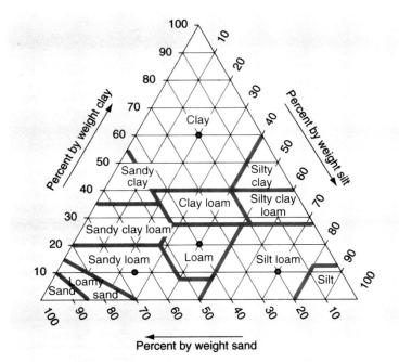
**Figure 4.3** Soil textural triangle used to identify the class of soil (taken from Miller and Gardner, 2001).
