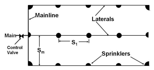
Figure 2.2 Example layout of single set required for this spray field.
