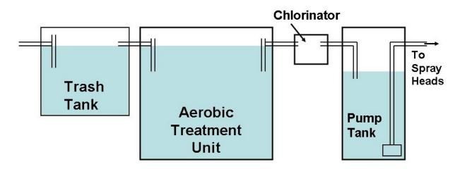
Figure 1.1. Diagram of a typical aerobic OSSF system with surface application of the effluent.
