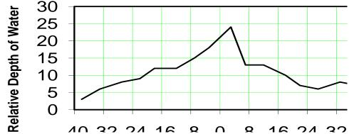
**Figure 6.1.** Typical shape of sprinkler pattern for an individual sprinkler. Sprinkler is located at the zero point on the graph.
