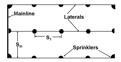
Figure 2.1. Example layout of a sprinkler system with a 30 ft by 30 ft head spacing and the 8 blocks required.
