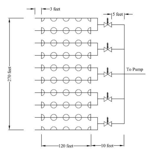
Figure 2.2. Layout of the sets for the spray field (not to scale).
