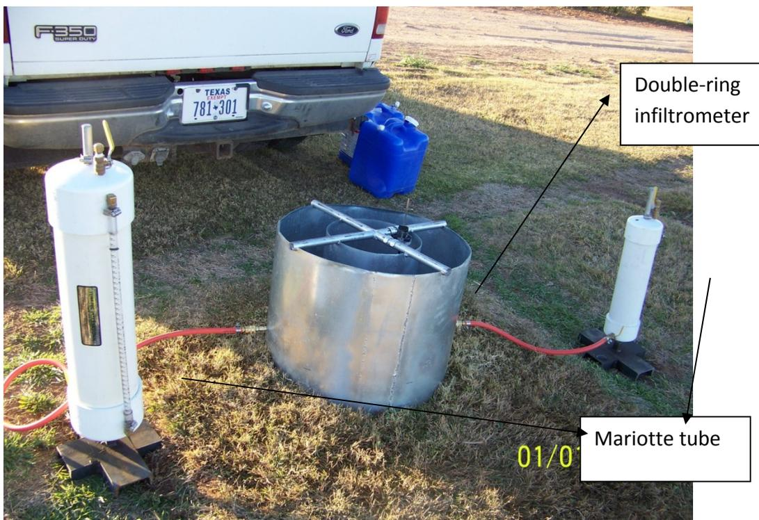
**Figure 4.** Double-ring infiltrometer and Mariotte tubes used in the standard ASTM infiltration tests.
