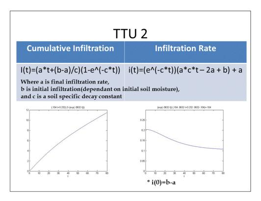
Figure 13. Boundary conditions for the TTU2 equation.
