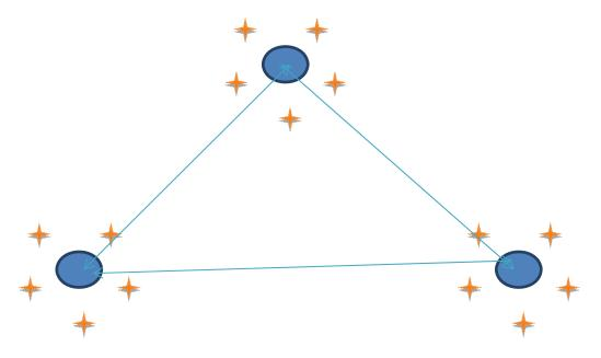
**Figure 9.** Layout of soil samples collected at each location. Circles represent the infiltrometer while the + represents the location of soil samples.
