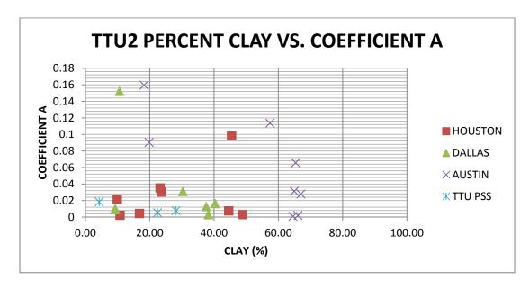
**Figure 15.** Relationship between the "A" coefficient from the TTU2 Equation and the percent clay content of the soil for all site locations with the outlier data removed.
