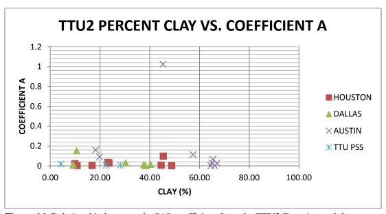
**Figure 14.** Relationship between the "A" coefficient from the TTU2 Equation and the percent clay content of the soil for all site locations.
