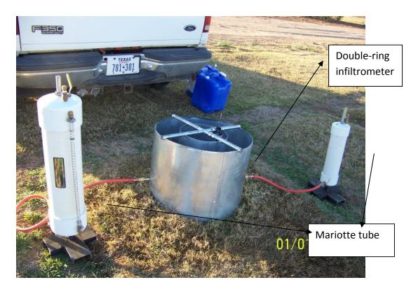
**Figure 4.** Double-ring infiltrometer and Mariotte tubes used in the standard ASTM infiltration tests.
