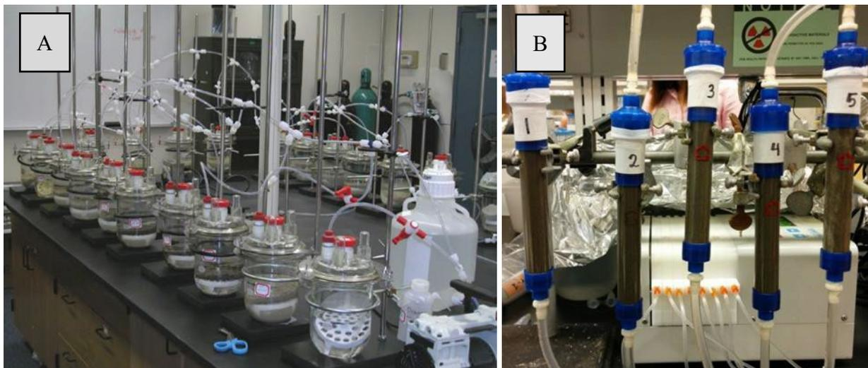
Figure 8A. Batch reactors with nitrogen gas lines (from Arthur et al., 2008)
