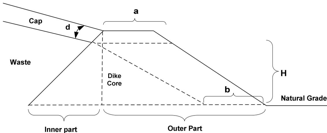
The base width of the erosion-critical portion may be calculated for a Class 1 landfill as  $b = 6/H$ , and for a Class 2 landfill as  $b = 5/H$ , where  $b$  is the base width and  $H$  is the height to the top of the cap over the dike. The erosion-critical portion should be constructed of clean soils that will support vegetation and that will resist erosion. If available, a soil with a lower erosivity than clay should be used with this design.
