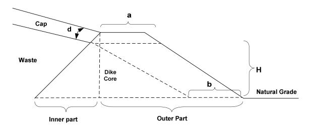
The base width of the erosion-critical portion may be calculated for a Class 1 landfill as b = 6/H, and for a Class 2 landfill as b = 5/H, where b is the base width and H is the height to the top of the cap over the dike. The erosion-critical portion should be constructed of clean soils that will support vegetation and that will resist erosion. If available, a soil with a lower erosivity than clay should be used with this design.
