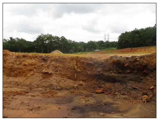
Figure 35: Truncated Weches Formation at ground surface with no remaining Holocene unit
