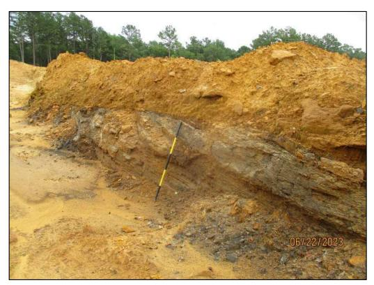
Figure 36: View of truncated Weches Formation below mechanical push pile
