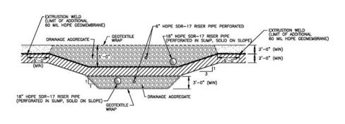
TYPICAL LEACHATE/UNDERDRAIN SUMP SECTION (UD1
