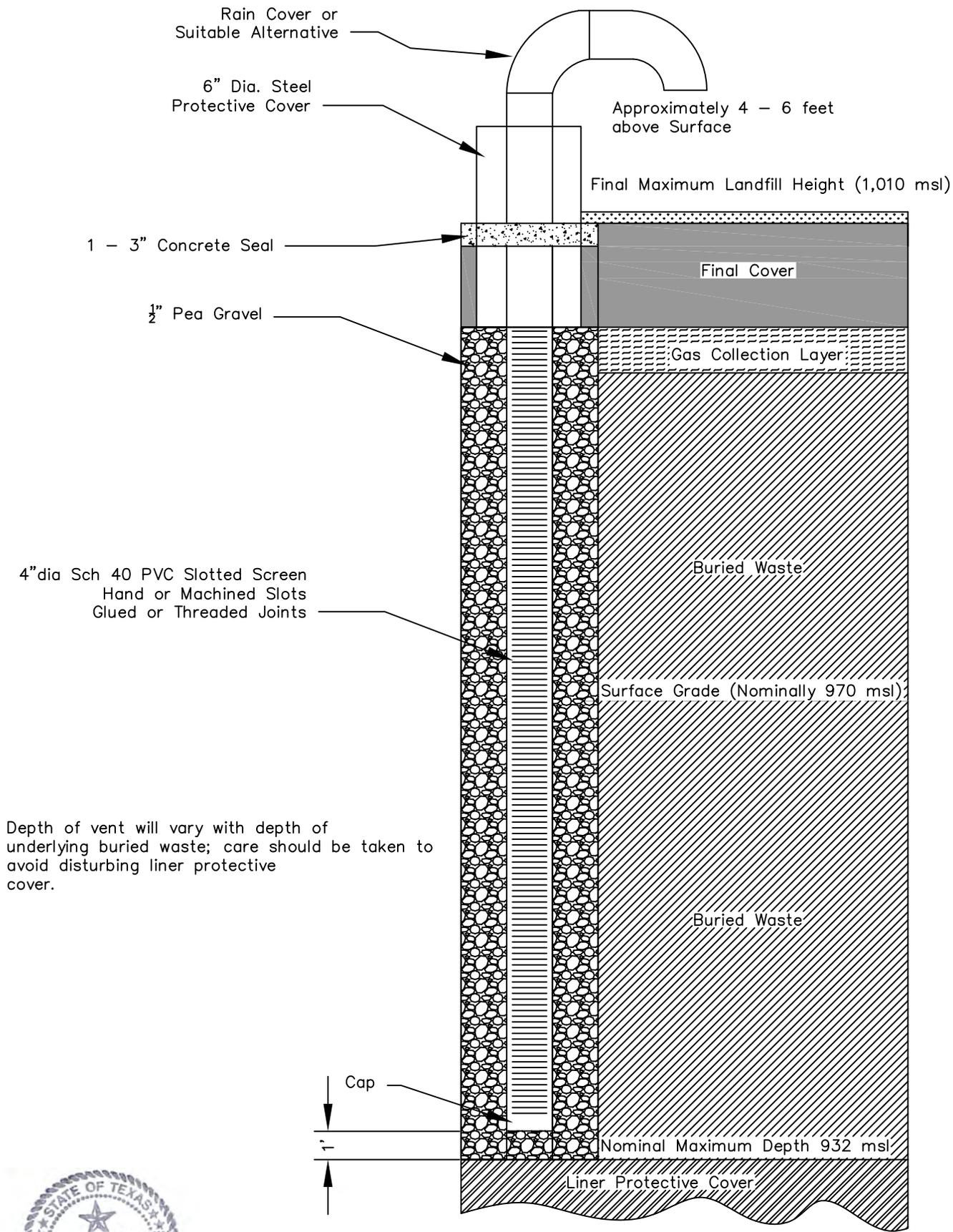
Depth of vent will vary with depth of underlying buried waste; care should be taken to avoid disturbing liner protective cover.
