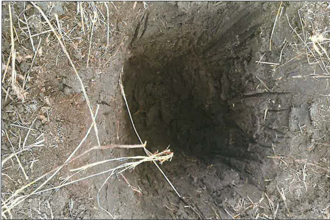
Figure 17. A typical shovel test (ST 07) from the project area, showing compact, dark gray (10YR 4/1) clay. Photograph taken May 2, 2025.
