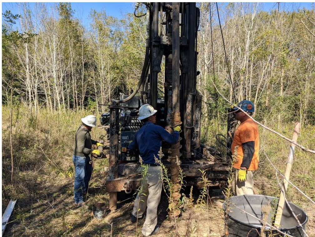
Hollow Stem Auger on Closed City of Bellaire Landfill
