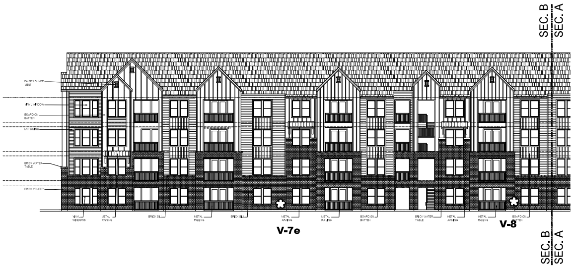
02 BUILDING 'A' EAST ELEVATION SCALE: 3/32" = 1'-0"
