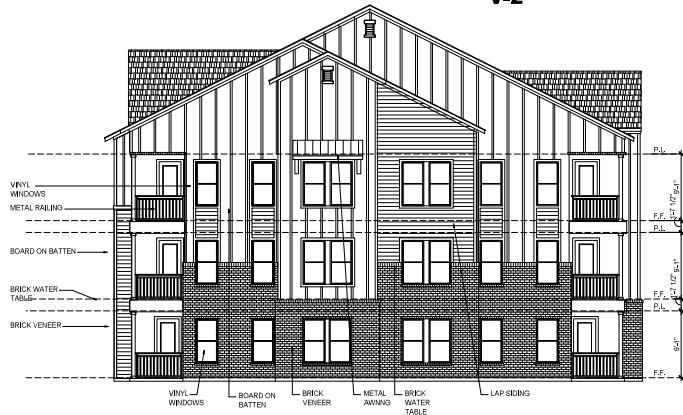
03 BUILDING 'D' LEFT ELEVATION SCALE: 1/8" = 1'-0"
