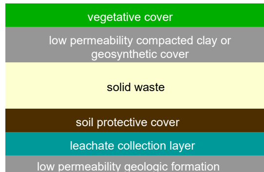
Figure 2.1 The liner and cover systems are designed to meet or exceed all state and federal regulations.
