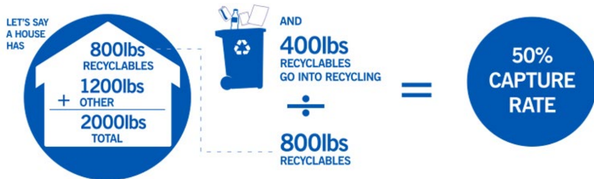
Figure 11: Example Capture Rate Calculation
