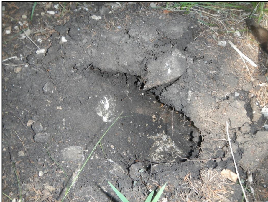
Figure 5. Overview of typical soil composite sample profile; note degrading bedrock at base.
