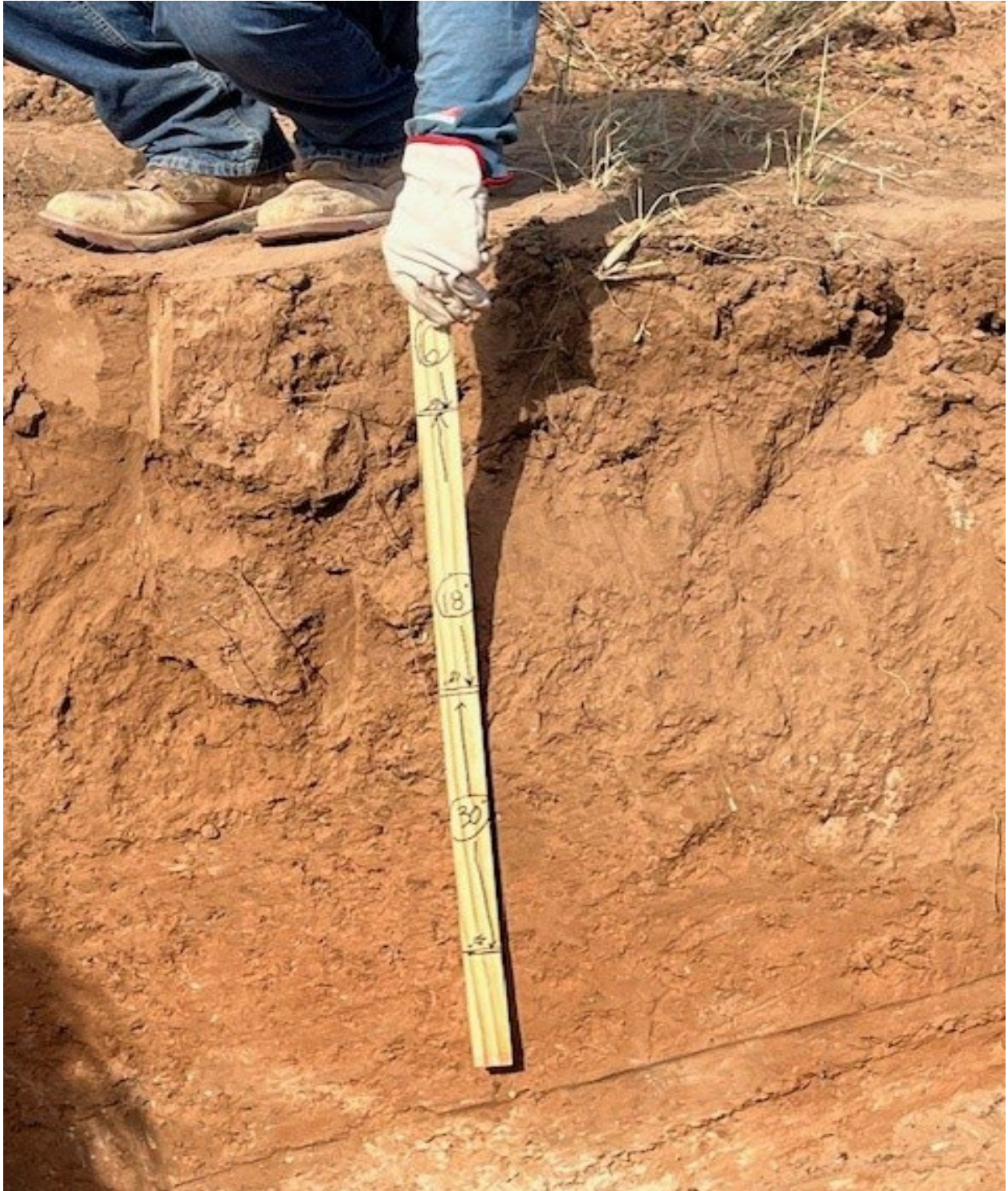
Photo 1 – Trench 6 showing soil profile and 0-6", 6"-18" and 18"-30" sample intervals. Total depth 6 feet below ground surface
