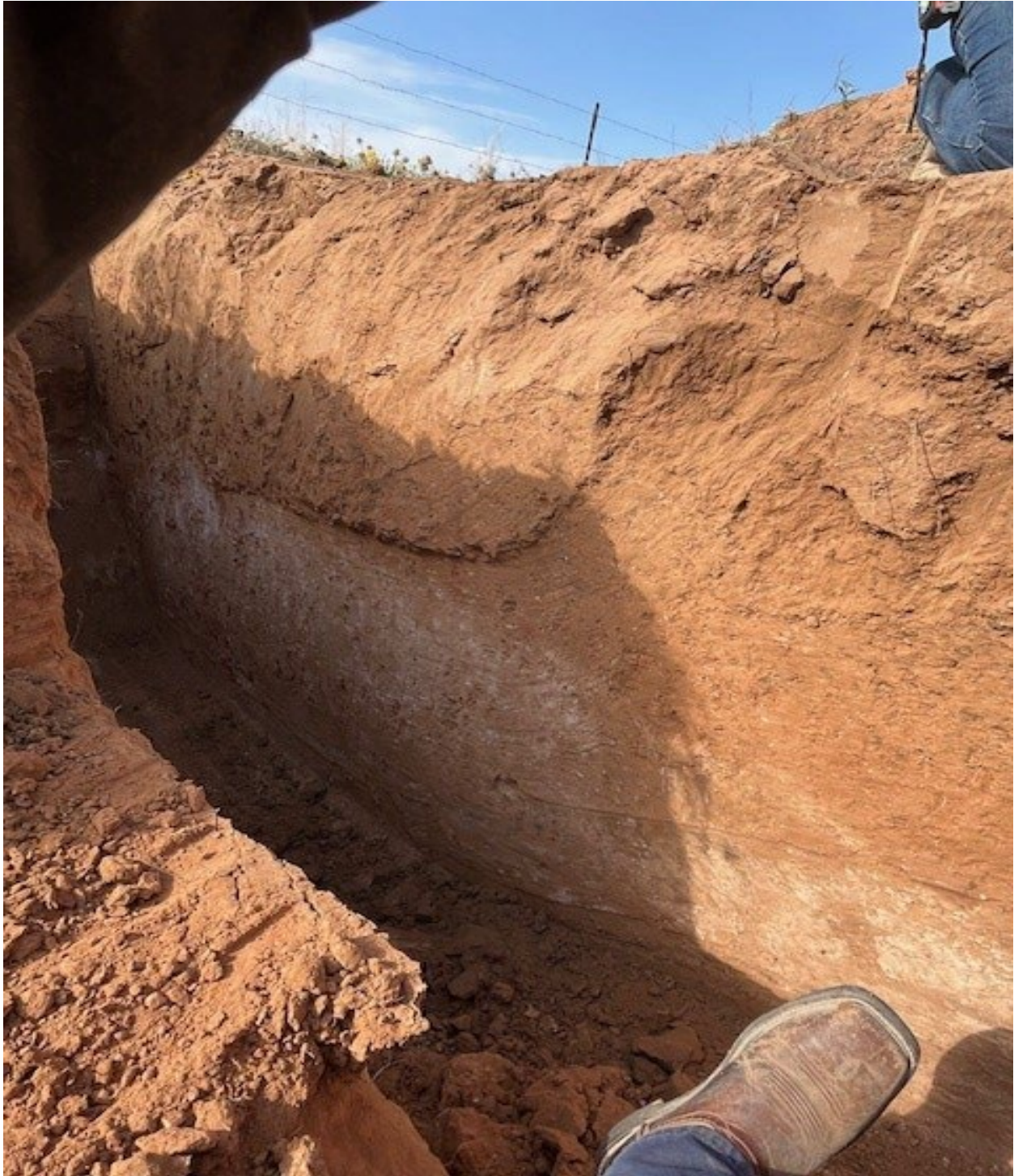
Photo 2 – Trench 6 view facing southwest showing transitory formation of calcium carbonate ( \text{CaCO}_3 ) in silty sands at depths of 3 to 4 feet. The \text{CaCO}_3 soils were soft digging from 3-5 feet and becoming denser with depth to 6 feet.
