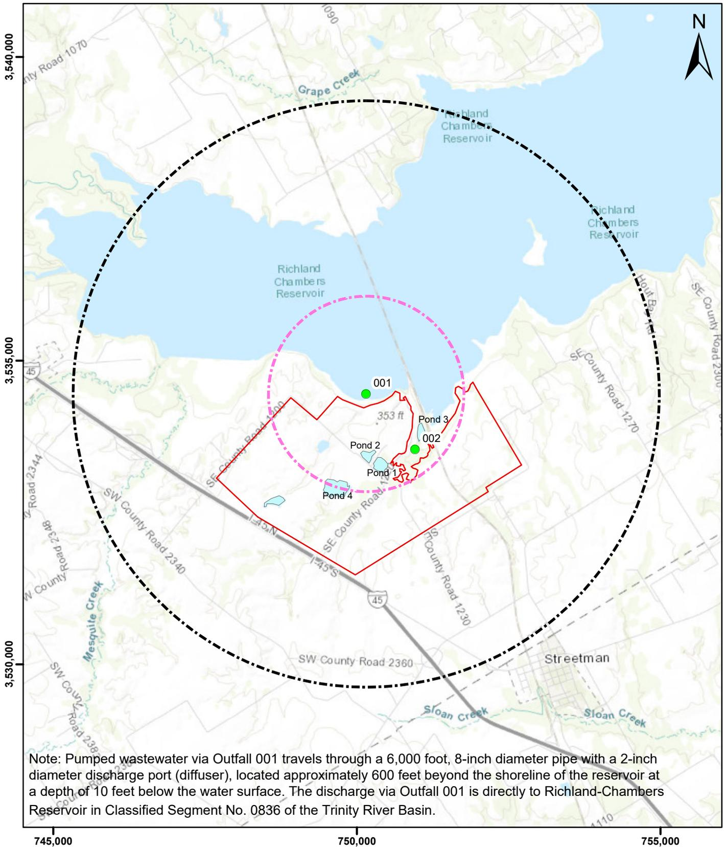
Note: Pumped wastewater via Outfall 001 travels through a 6,000 foot, 8-inch diameter pipe with a 2-inch diameter discharge port (diffuser), located approximately 600 feet beyond the shoreline of the reservoir at a depth of 10 feet below the water surface. The discharge via Outfall 001 is directly to Richland-Chambers Reservoir in Classified Segment No. 0836 of the Trinity River Basin.
