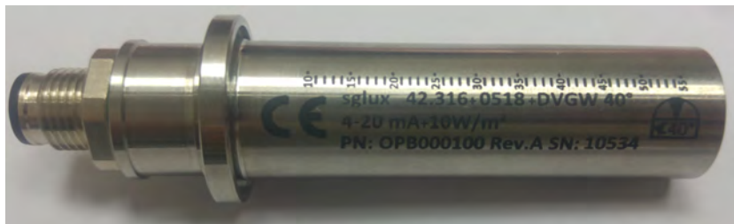
Figure 10-25: Sensor casing, showing millimeter scale
