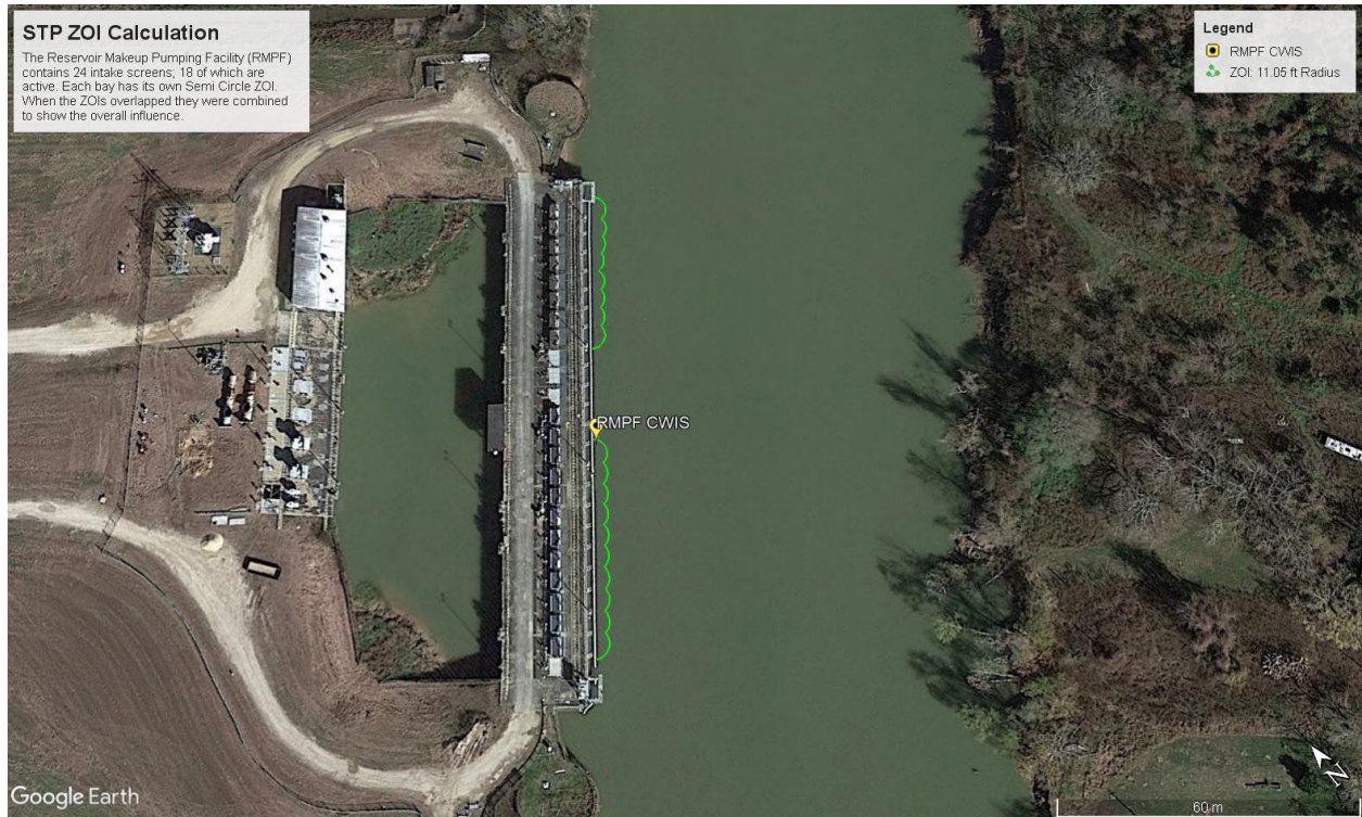
FIGURE 11: Expected Zone of Influence at the RMPF Cooling Water Intake Structure
