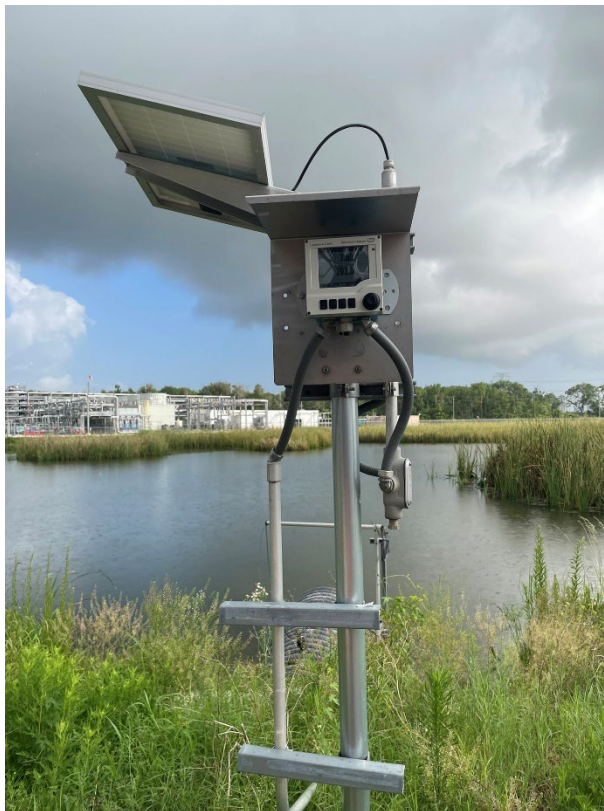
Photo 4 – Pond exit pipe to Outfall 001 and pH/Temperature meter
