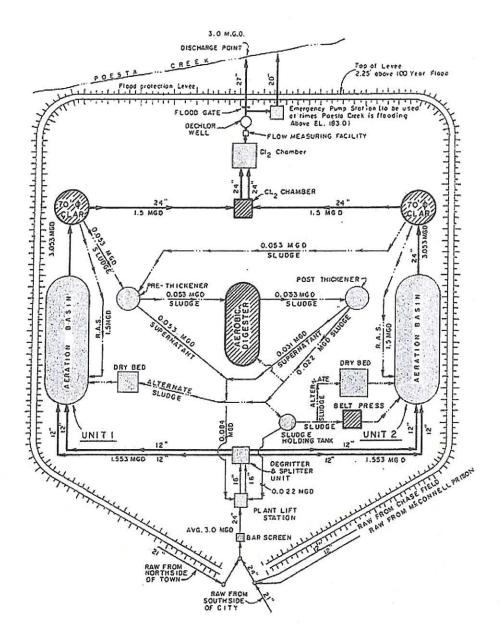
SCHEMATIC FLOW DIAGRAM
