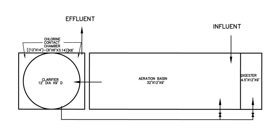
ATTACHMENT 4 TRI-COUNTY POINT PROPERTY OWNERS ASSOC. WASTEWATER TREATMENT PLANT FLOW DIAGRAM
