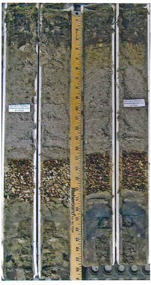
**Core Observations:** We received PVC tubes containing undisturbed soil profiles from the #13 green. The profiles were labeled either Good Middle Left or Bad Front Middle Low. We cut one Good core and one bad Core open lengthwise, exposing the entire profile. A photograph of the profiles is included to the left (Good Middle Left is the left photo).
