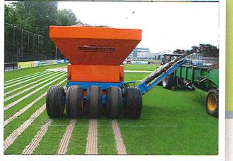
The DrainMaster has been developed to improve and accelerate surface water evacuation. Because of this, the stability and the quality of the turf will increase significantly. The DrainMaster digs three trenches at right
