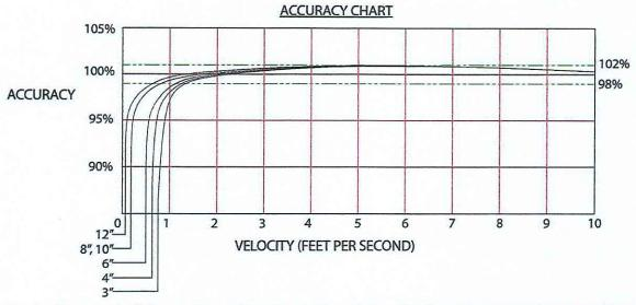
Standard flowrates for McCrometer propeller meters are shown below. Readings are guaranteed accurate within  $\pm 2\%$  in these flowrates. Please note that over 80 percent of the meter's flow range, the accuracy is better than  $\pm 1\%$ .
