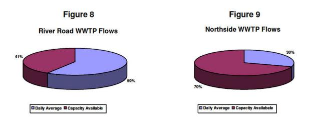
The City of Wichita Falls has prepared a Master Wastewater Plan that calls for the eventual construction of a new wastewater treatment plant at the time the maximum capacity of the River Road Wastewater Treatment Plant is neared. Conservation of water can play a major role in delaying the need for further expansion of collection and treatment facilities.
