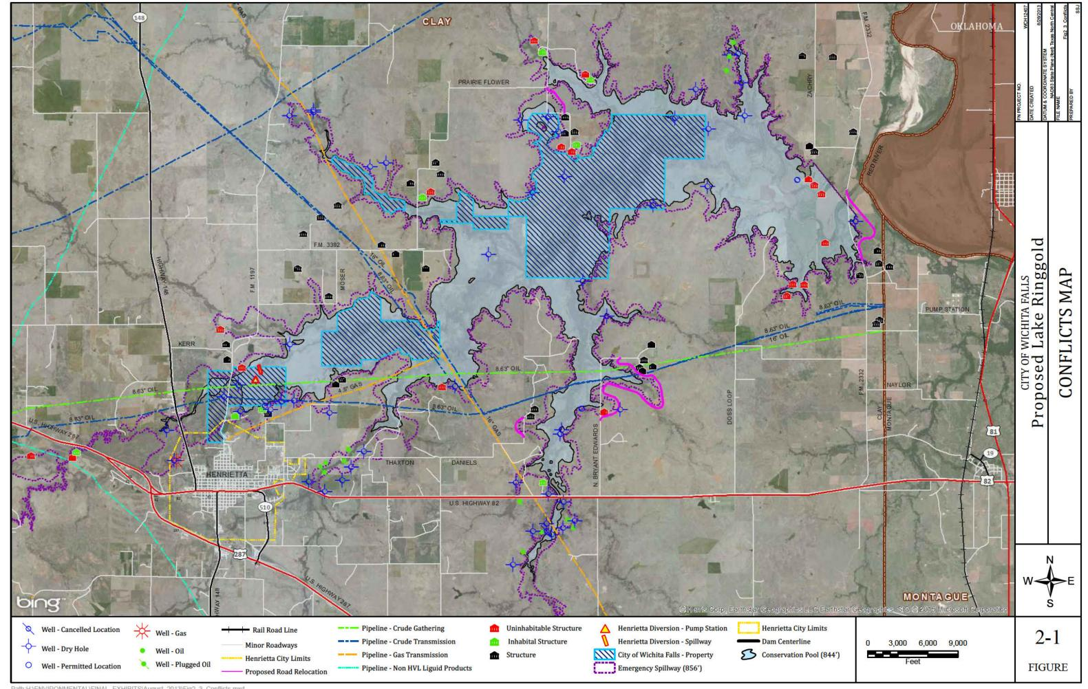
protected or moved. Within the acreage associated with the emergency spillway elevation, six additional residences and 17 additional structures may be impacted. Further site-specific investigations will be needed to confirm the elevations of these structures and appropriate resolution.
