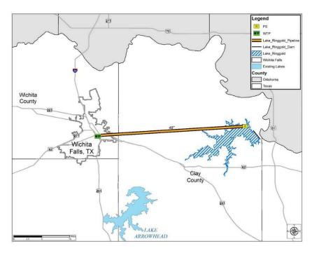
pipeline has not been determined. The alignment shown in Section 2.1 is for costing purposes only. One option would be to pump diverted water from Lake Ringgold to Lake Arrowhead, and then utilize existing and/or future transmission facilities to move the water to the City. The water would be treated at an existing water treatment plant.
