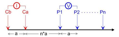
$C_a$  and  $C_b$  are the current electrodes and  $P_1$ ,  $P_2$  to  $P_n$  are the potential electrodes during measurements. The distance between the current electrode  $C_a$  and the potential electrode  $P_1$  is an integer multiple,  $P_n$ , of the distance between the current or potential electrode pair. For this study,  $P_n$  ranges from 1 to 6.
