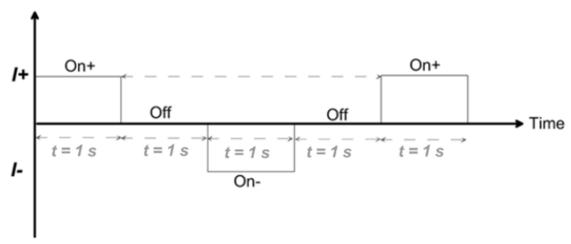
During induced polarization measurements, 20 IP windows were used to define the decay curve in the semi logarithmic mode when the current is shut off. In semi logarithmic mode, the first eight windows span a 20 millisecond (ms) interval per window. The following six measurement windows span 40 ms per window. The last six windows span 80 ms each. The time delay between current shut off and the beginning of the decay curve is 40 milliseconds.
