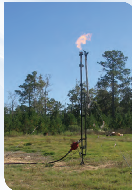
This is an example of an air-assisted flare effectively burning and destroying excess waste gas and achieving high efficiency. Notice the flame.
