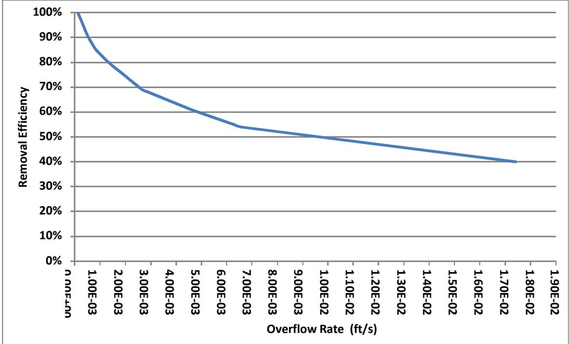
**Figure 3 Relationship between Removal Efficiency and Overflow Rate**
