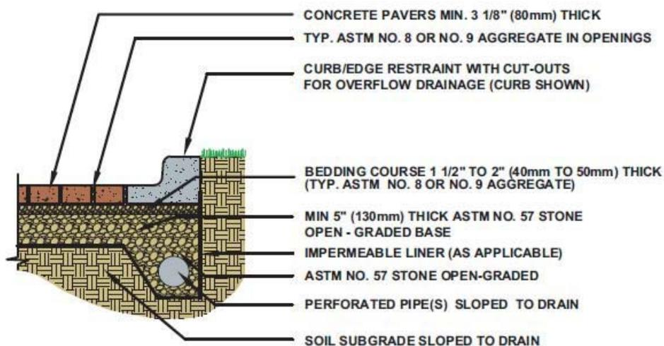
**Figure 7 Permeable Pavers – Vehicular**
