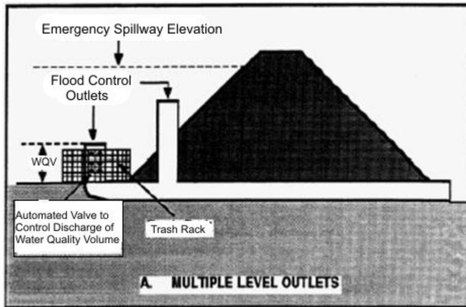
**Figure 3 Example of Configuration Combining Flood and Water Quality**
