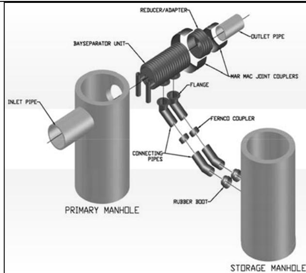
**Figure 5 Schematic of the BaySeparator System**
