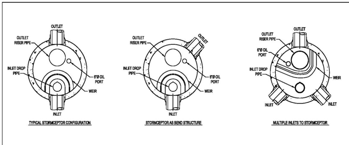
**Figure 2 Stormceptor® In-Line Configurations**
