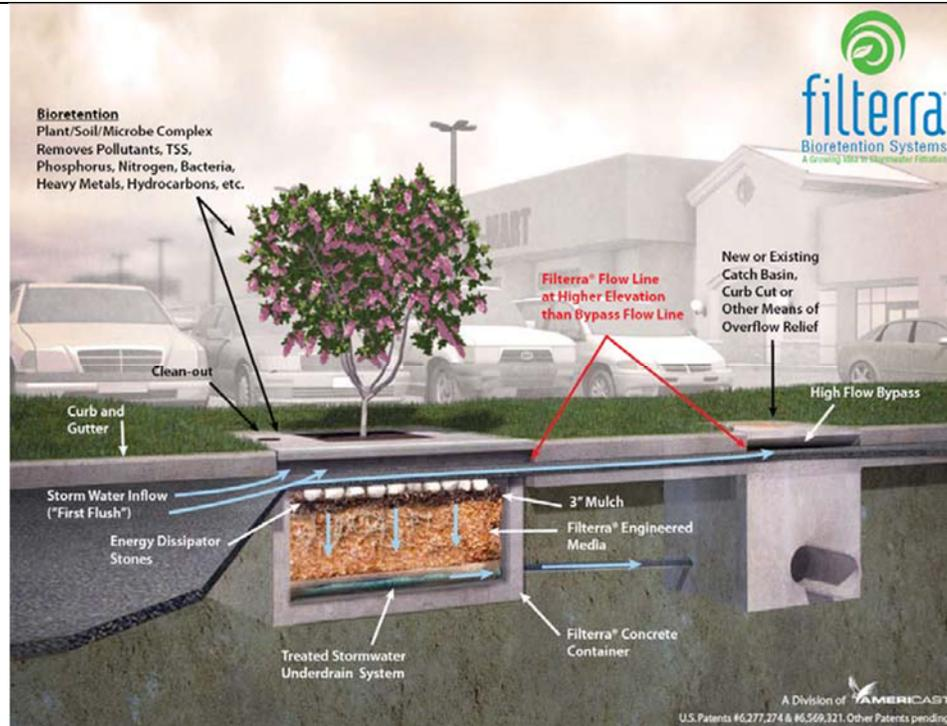
**Figure 1 Filterra® Schematic**
