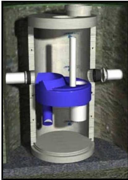
**Figure 3-33 Stormceptor® Diagram**
