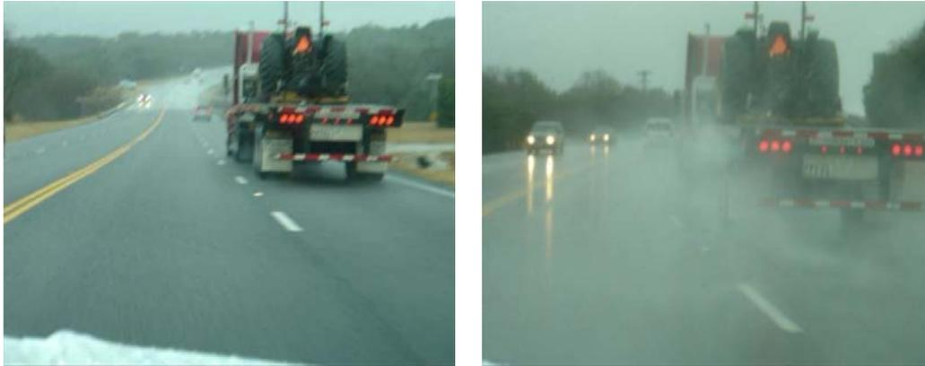
**Figure 1 Difference in Spray from Conventional and PFC Pavements**
