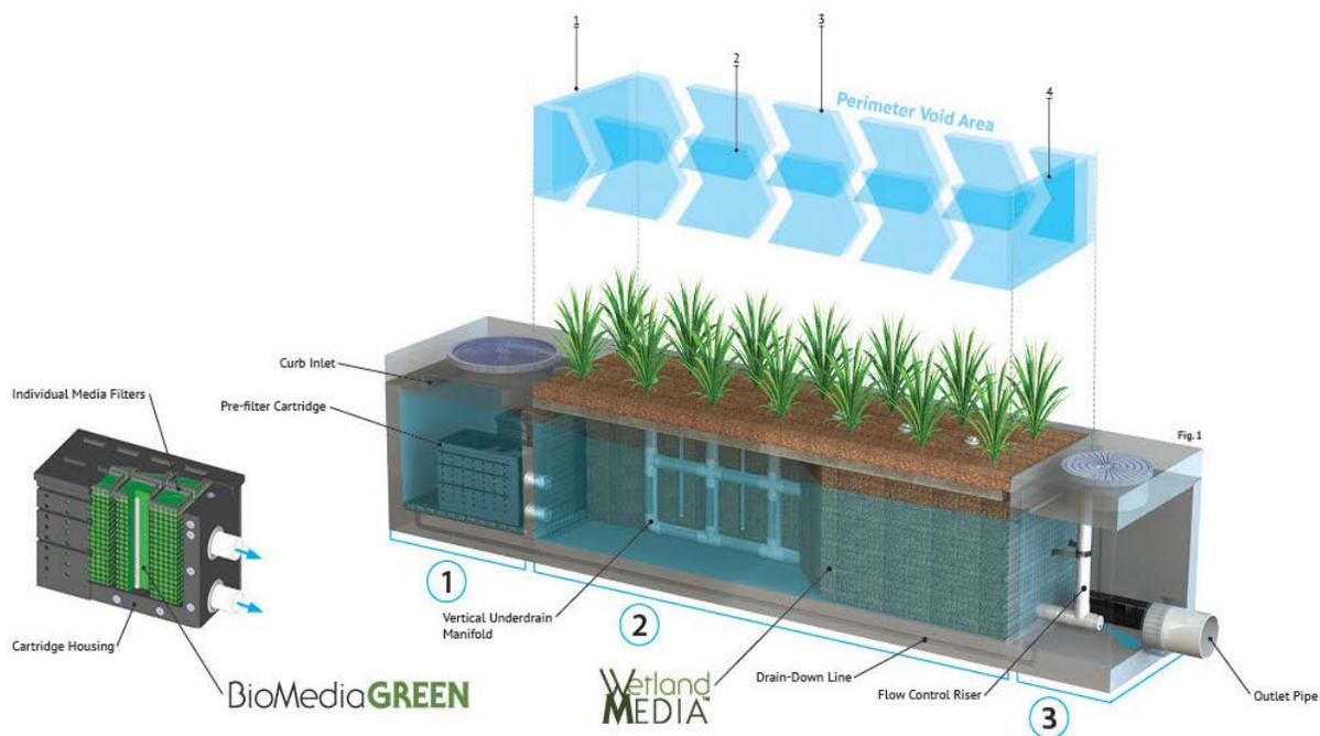
**Figure 1 MWS Linear Schematic**
