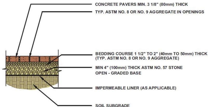
**Figure 6 Permeable Pavers – Pedestrian**
