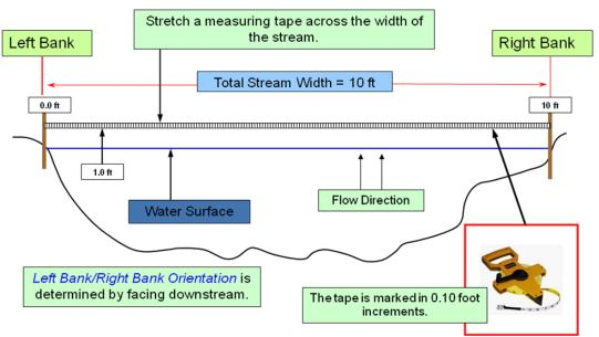
Figure 3.6. Measuring the stream width.
