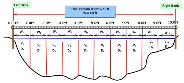
Figure 3.15. Streamflow (discharge) measurement.
