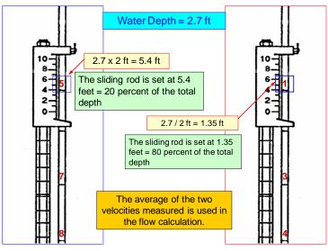
Figure 3.12. Setting the flow sensor at depths > 2.5 feet.
