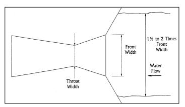
Figure 3.36. Top view of the cutthroat flume (Baski, Inc.).
