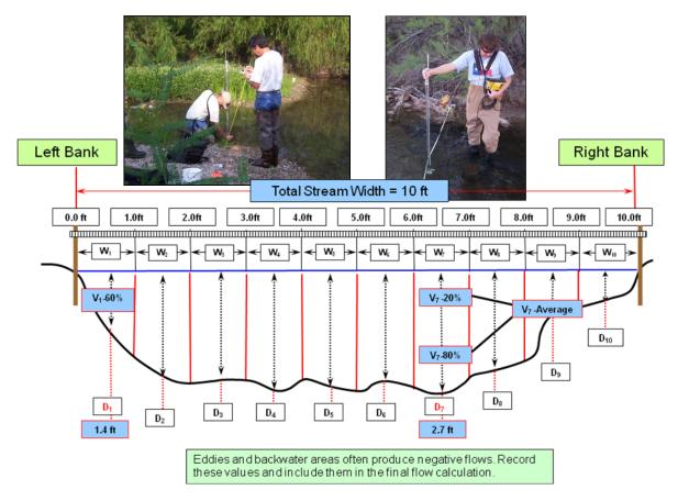
Figure 3.13. Measuring velocity.
