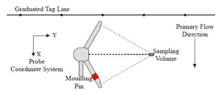
Figure 3.28. FlowTracker probe orientation relative to streamflow.
