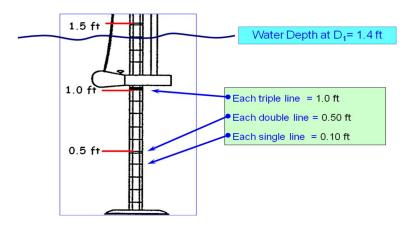
Figure 3.9. Measuring the depth using a top-setting wading rod.
