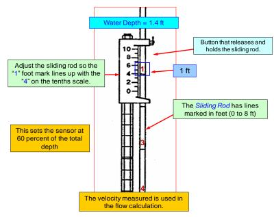
**Figure 3.11.** Setting the flow sensor at depths  $\leq 2.5$  feet.
