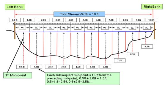
Figure 3.7. Determining the midpoint of the cross-section.
