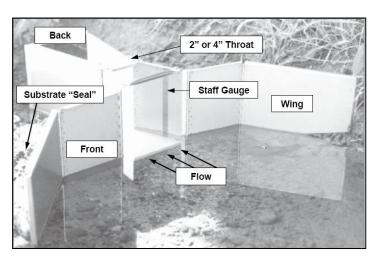
Figure 3.35. Portable cutthroat flume (Baski, Inc.).
