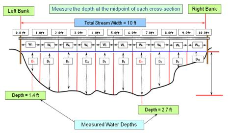
Figure 3.8. Measuring the depth at each midpoint.
