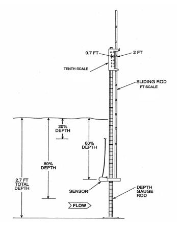
Figure 3.10. Top-setting wading rod.
