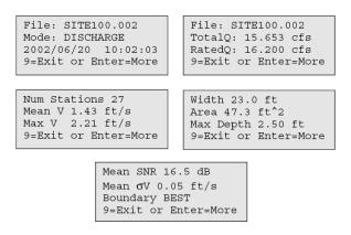
Figure 3.27. Final Discharge Measurement screens.
