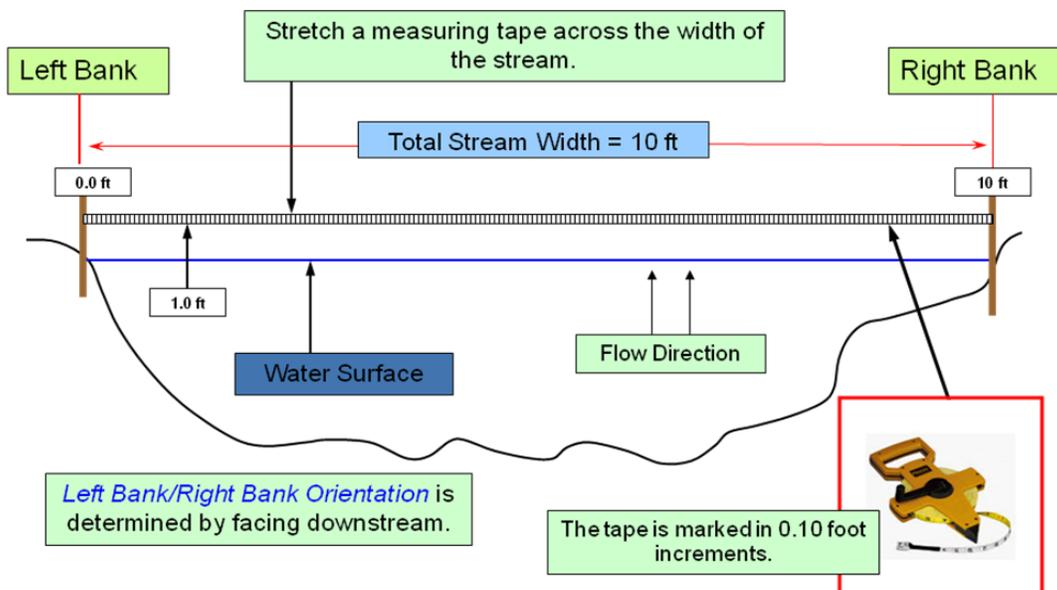
**Figure 3.6.** Measuring the stream width.
