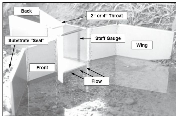
Figure 3.35. Portable cutthroat flume (Baski, Inc.).
