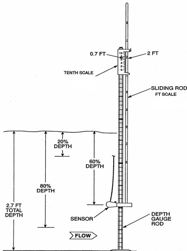
**Figure 3.10.** Top-setting wading rod.
