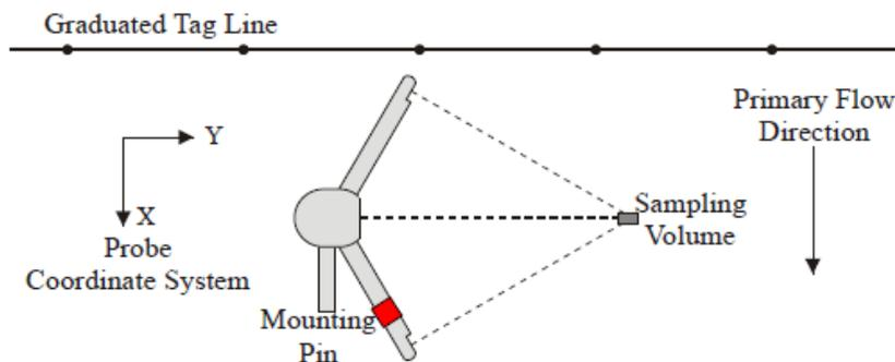
**Figure 3.28.** FlowTracker probe orientation relative to streamflow.
