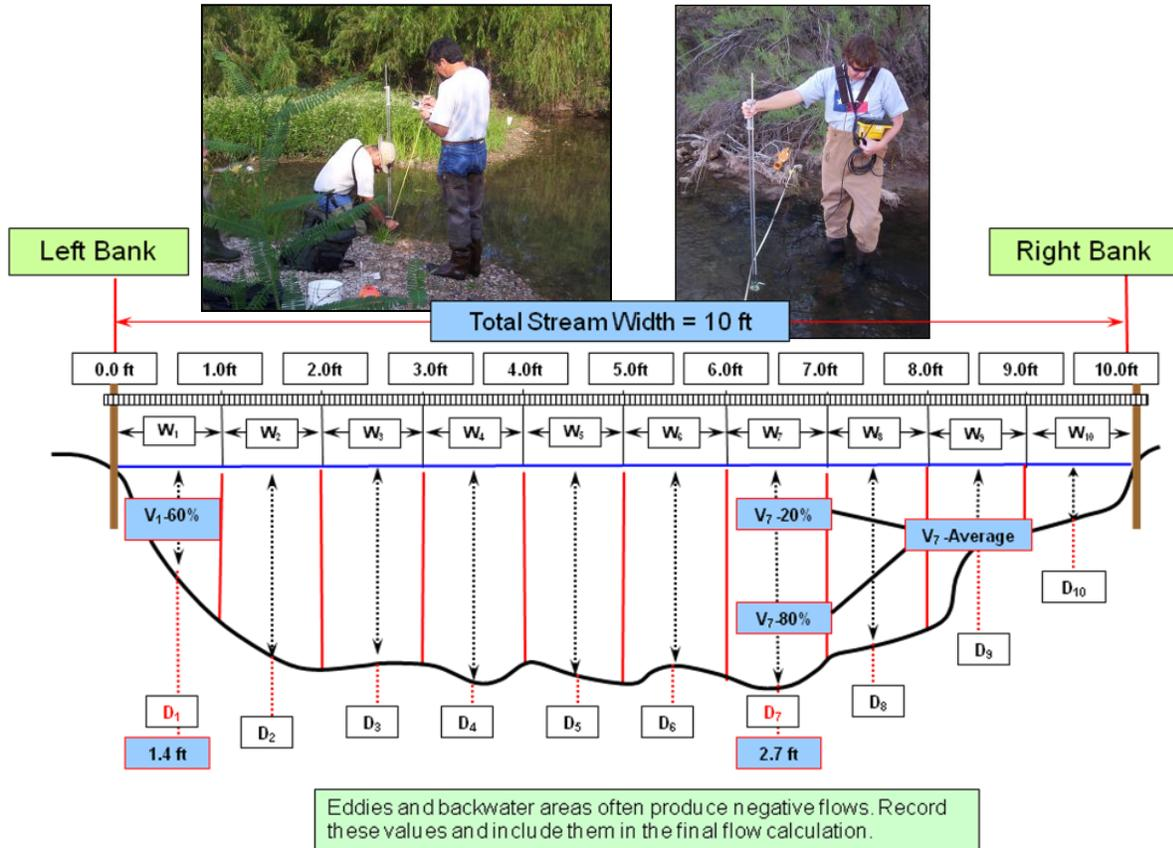
**Figure 3.13.** Measuring velocity.
