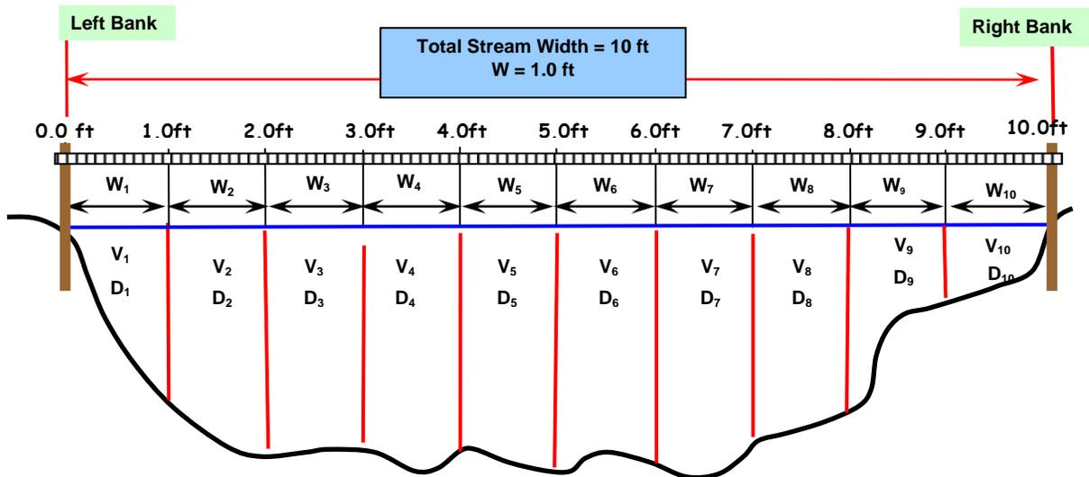
Figure 3.15. Streamflow (discharge) measurement.
