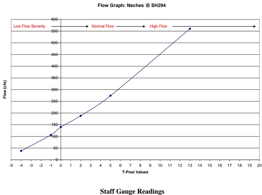
**Figure 3.38.** Staff gauge established at low flow.
