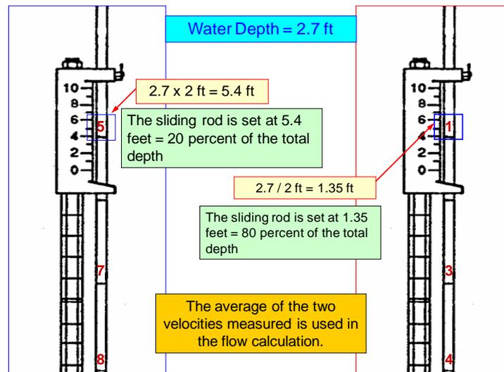
**Figure 3.12.** Setting the flow sensor at depths  $> 2.5$  feet.
