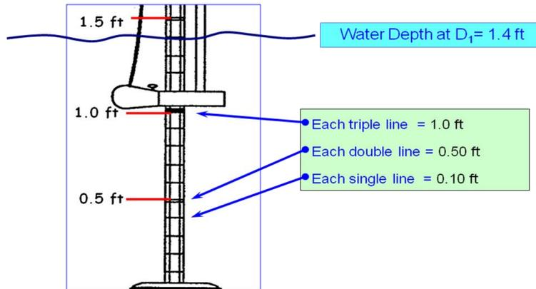
**Figure 3.9.** Measuring the depth using a top-setting wading rod.
