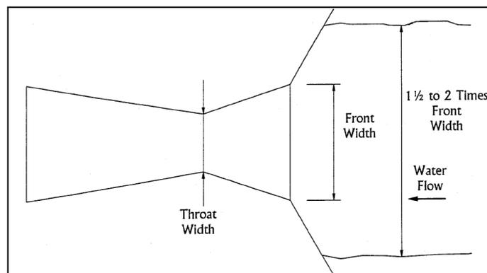
Figure 3.36. Top view of the cutthroat flume (Baski, Inc.).
