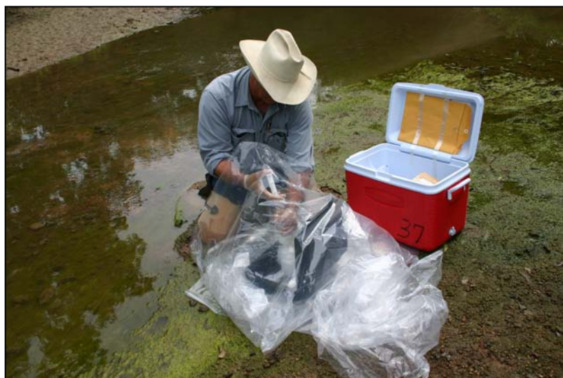
Figure 5.2. Collecting a dissolved-metals sample with a TCEQ Clean Metals Kit.
