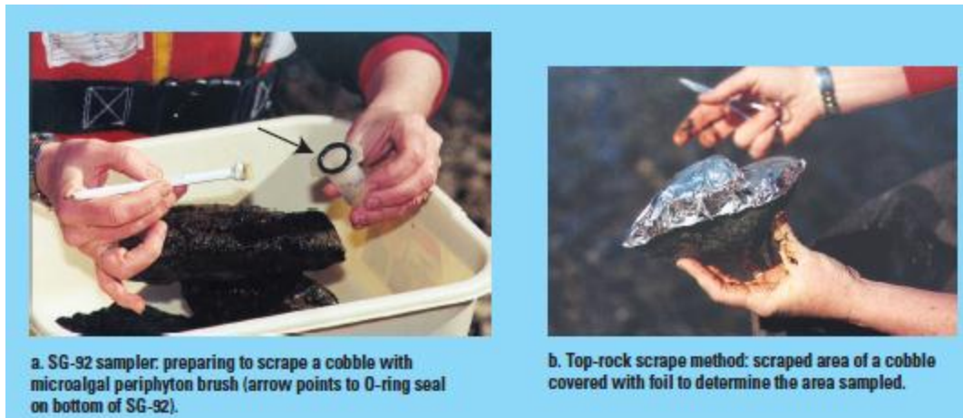
Figure 7.2. How to remove algae from rock surface and how to measure rock surface area. (USGS 2002.)
