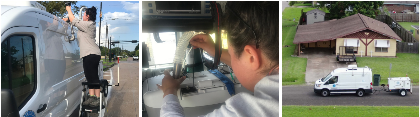
(Left and center) In the wake of Hurricane Laura, TCEQ deployed air quality monitoring vans equipped with rapid assessment survey technology, which reports air quality data in real-time. (Right) TCEQ staff drive a mobile-monitoring van through a neighborhood after Hurricane Laura.
