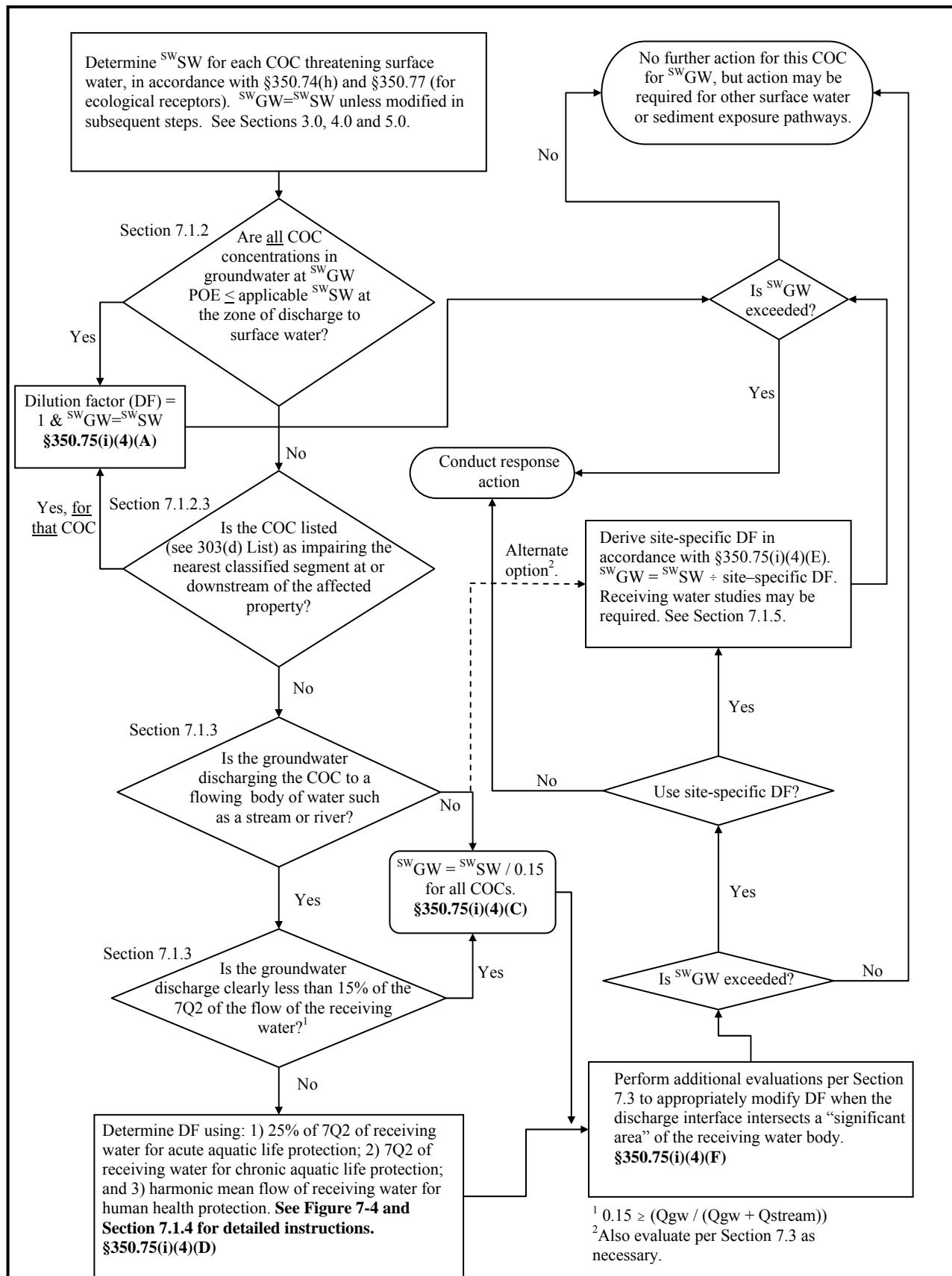
Figure 7-1. Determining the Groundwater-to-Surface Water Dilution Factor
