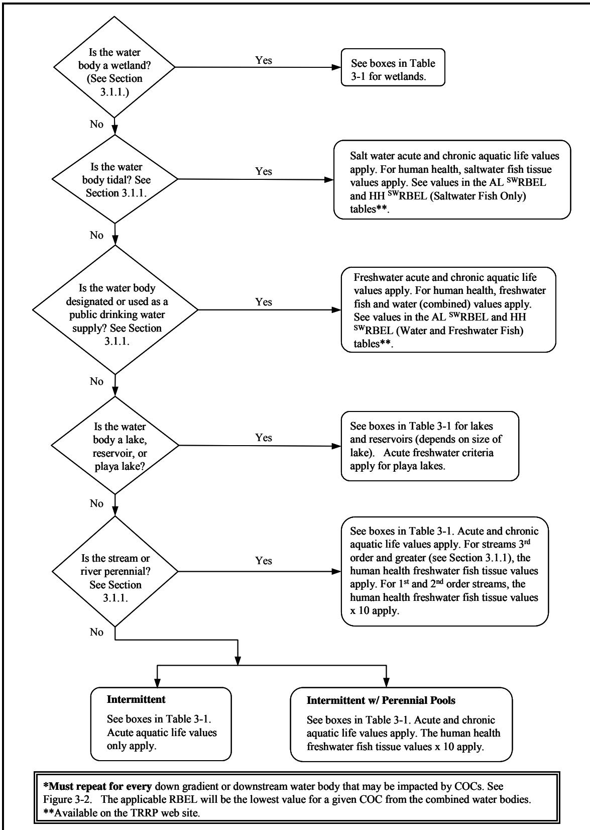
Figure 3-3. Determining the Applicable Water Quality Values Based on Water Body Type
