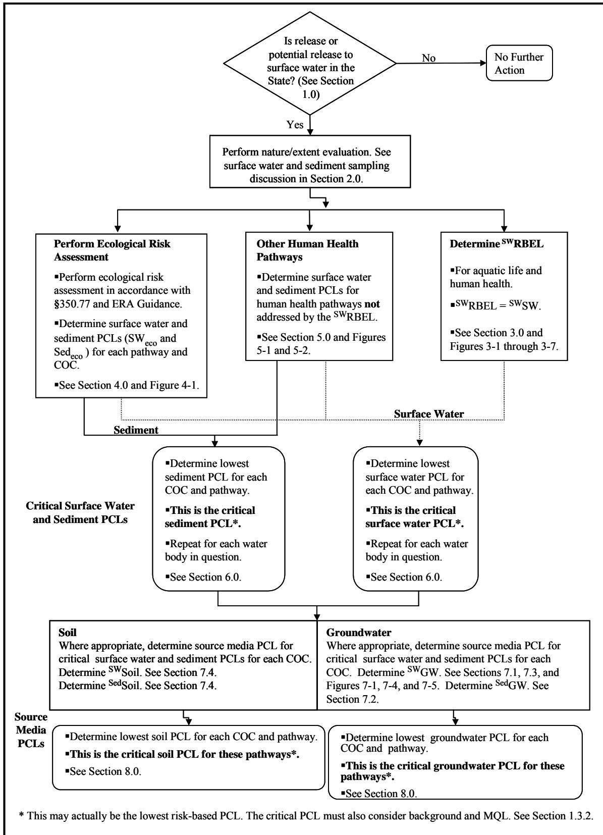
**Figure 1-1. Overview of the Process for Deriving Surface Water and Sediment PCLs**
