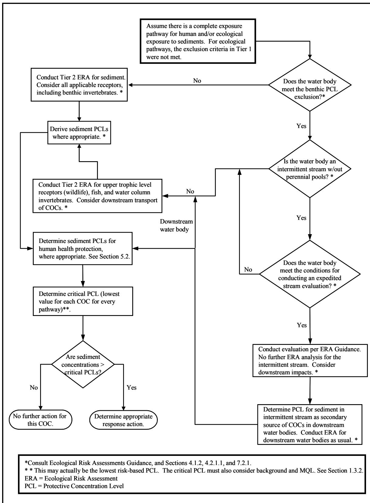
Figure 4-1. Determination of the Sediment PCL
