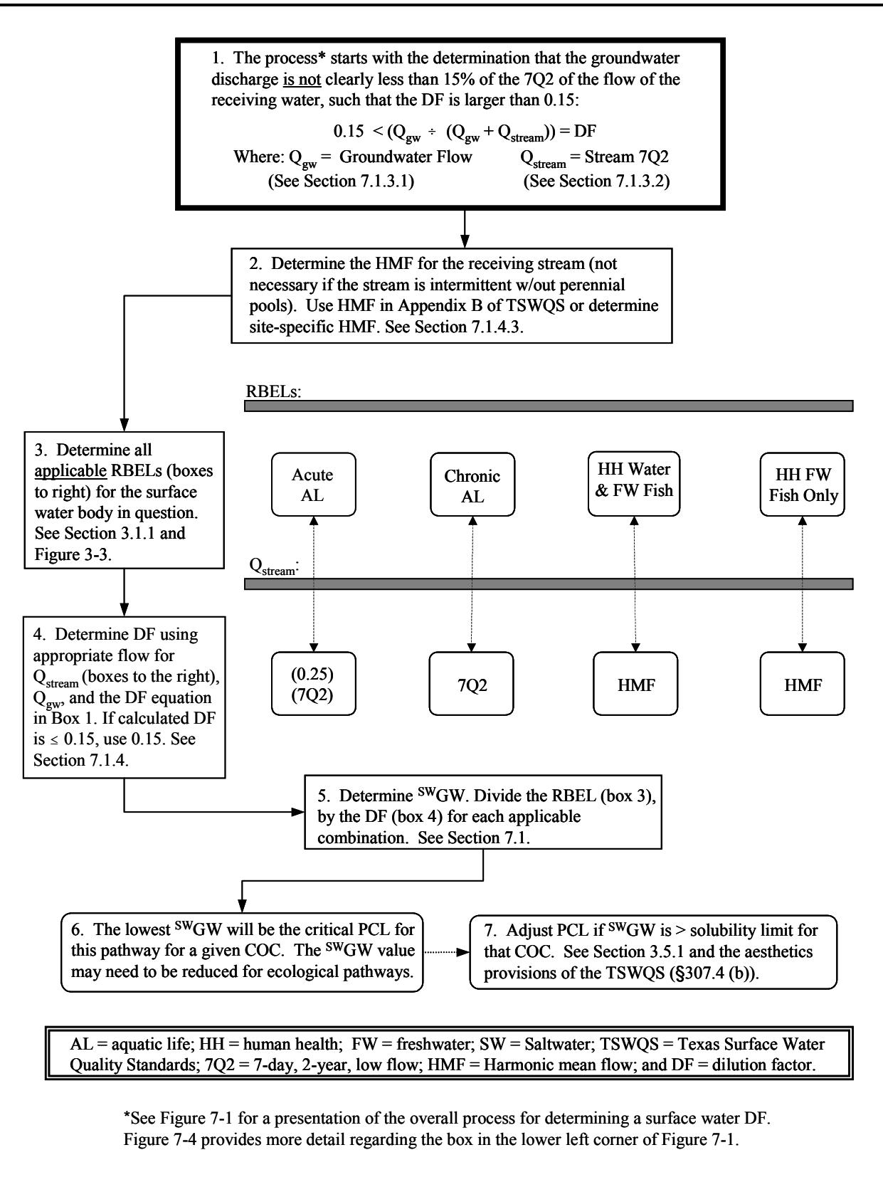
**Figure 7-4. Determining the  $^{sw}GW$  per 30 TAC §350.75 (i)(4)(D)**
