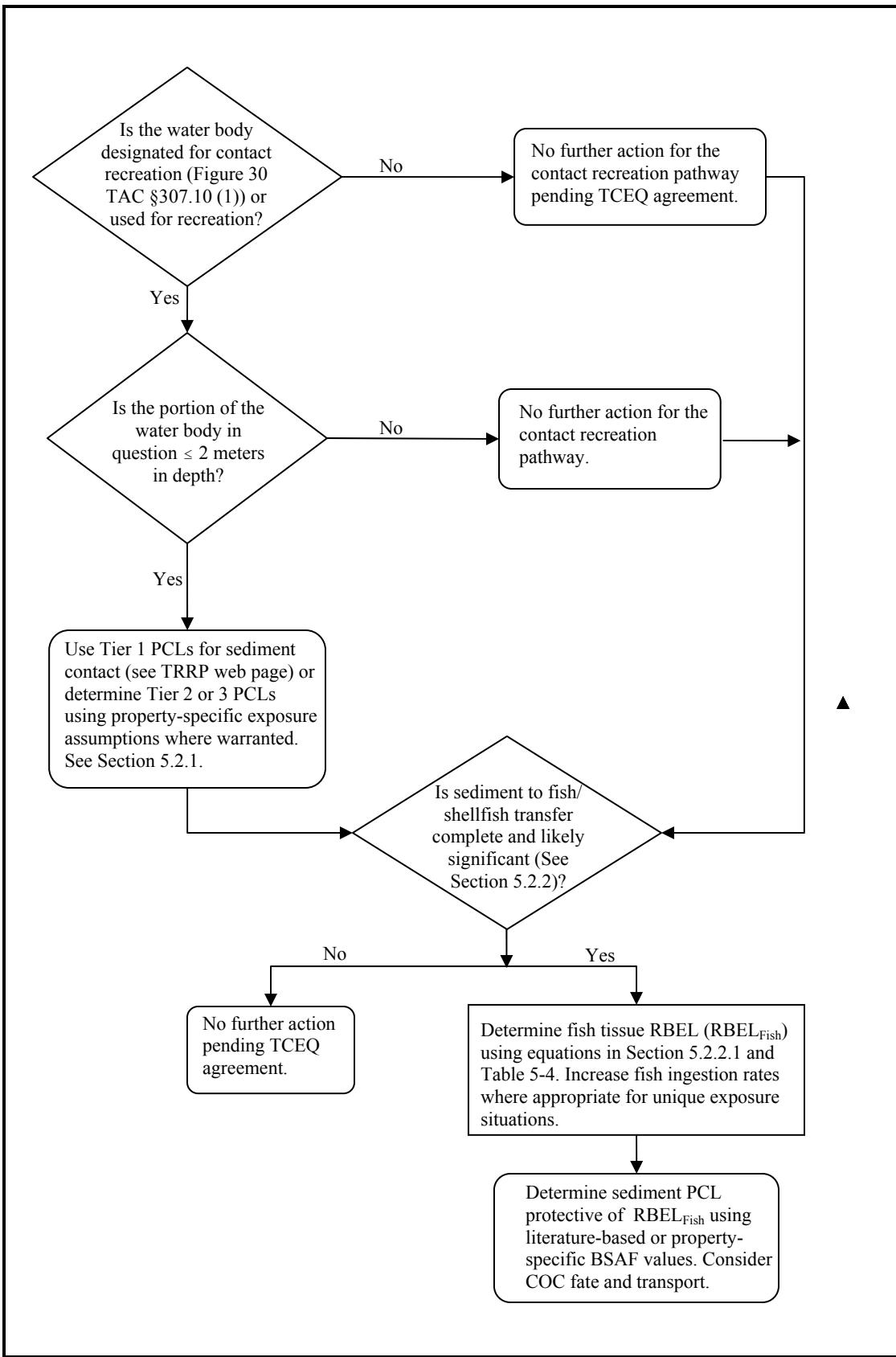
**Figure 5-2. Determining Sediment PCLs Protective of Human Health**
