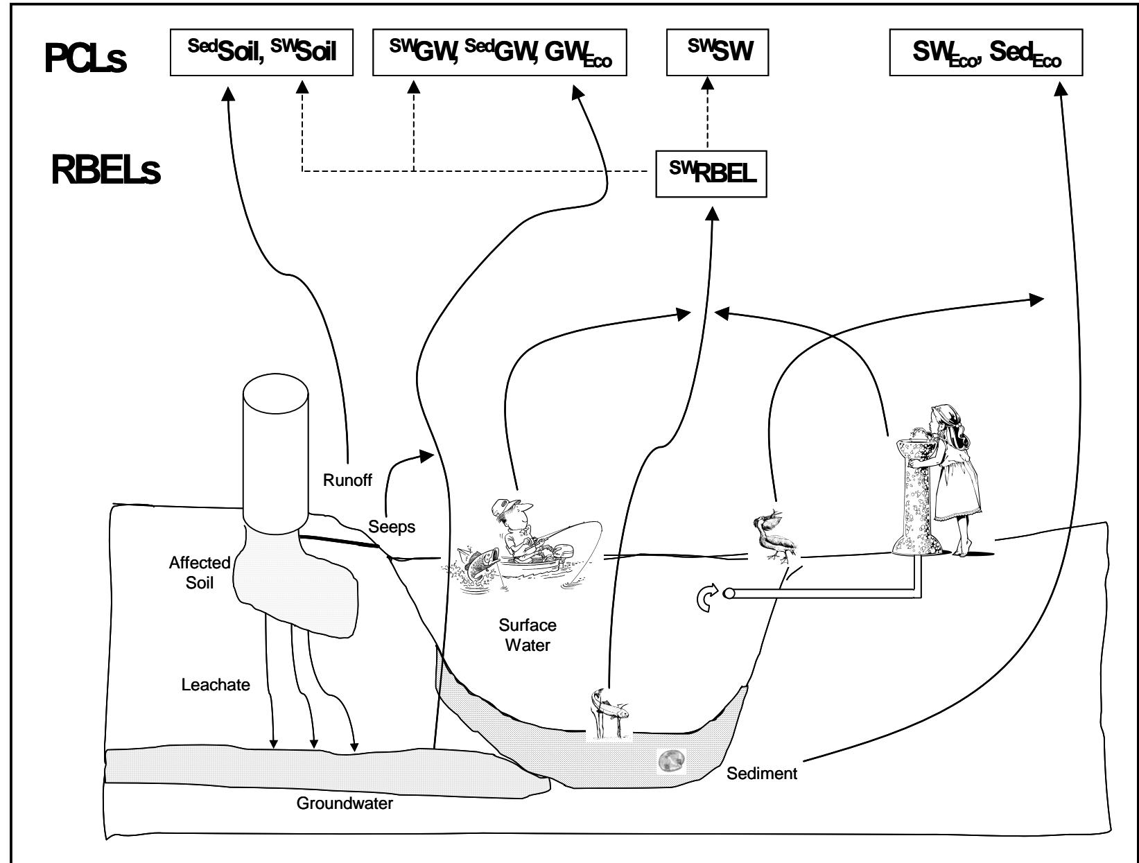
Figure 1-2. Surface Water and Sediment PCLs and RBELs
