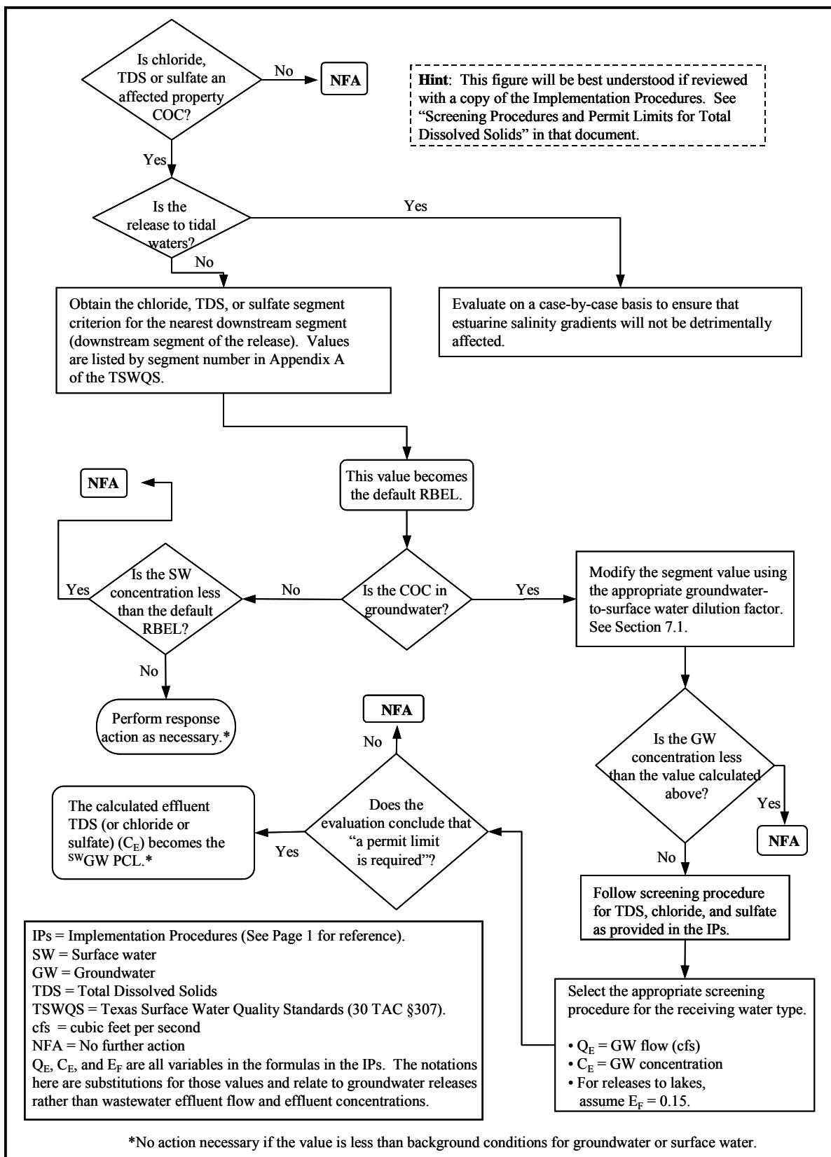
**Figure 3-6. Determining the  $^{SW}RBEL$  and  $^{SW}GW$  for TDS, Chloride, and Sulfate**
