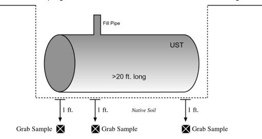
Figure 5. Tank-Hold Sampling: No Water Present, Tanks Greater than 20 ft in Length
