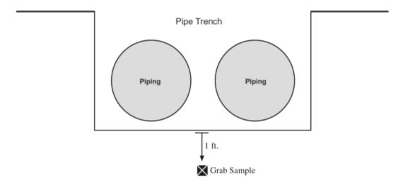
Figure 9. Pipe-Trench Sampling (Plan View)
