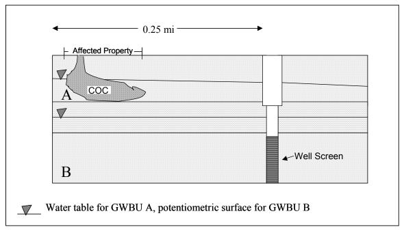
Figure 2. Hydrostratigraphic Scenario for Multiple GWBU Classification Example.
