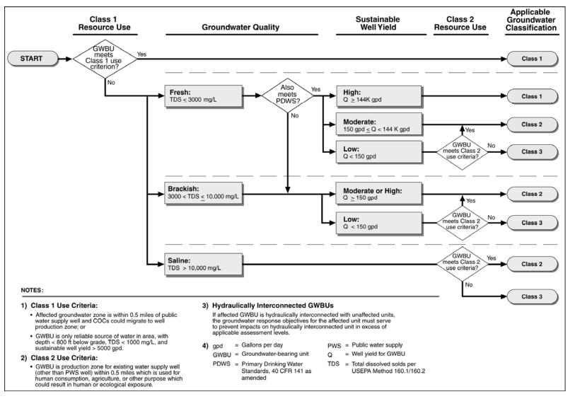
Figure 1. TCEQ Groundwater Resource Classification Logic Diagram.
