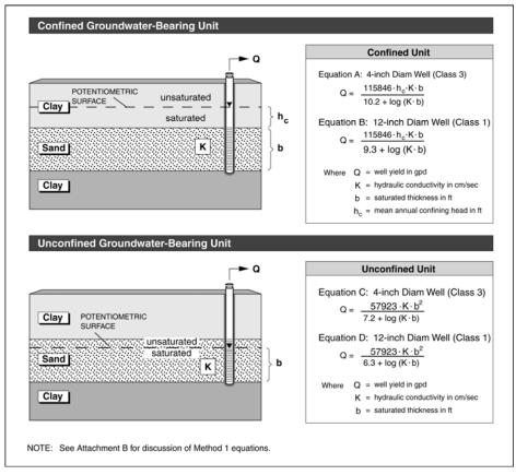
Figure 4. Method 1 Equations for Estimating Well Yield.
