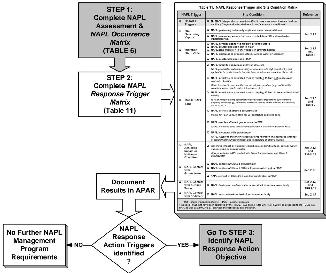
Figure 4. Overview of STEP 2: Identify NAPL Response Triggers.
