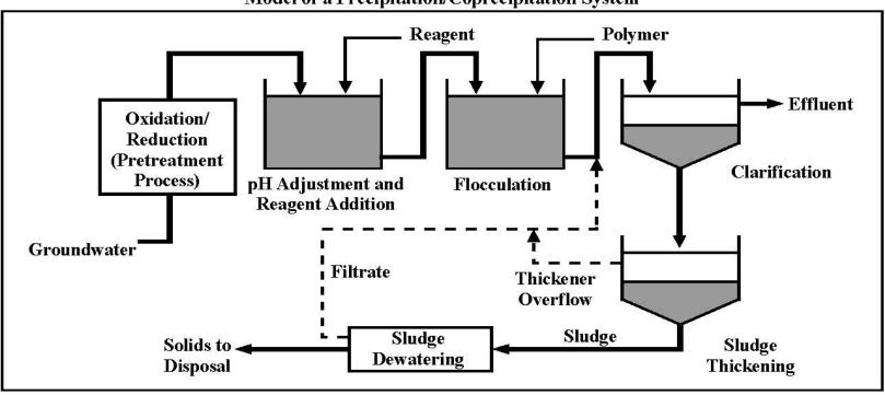
Model of a Precipitation/Coprecipitation System
