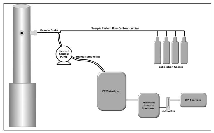
Figure 1: Sample System Diagram
