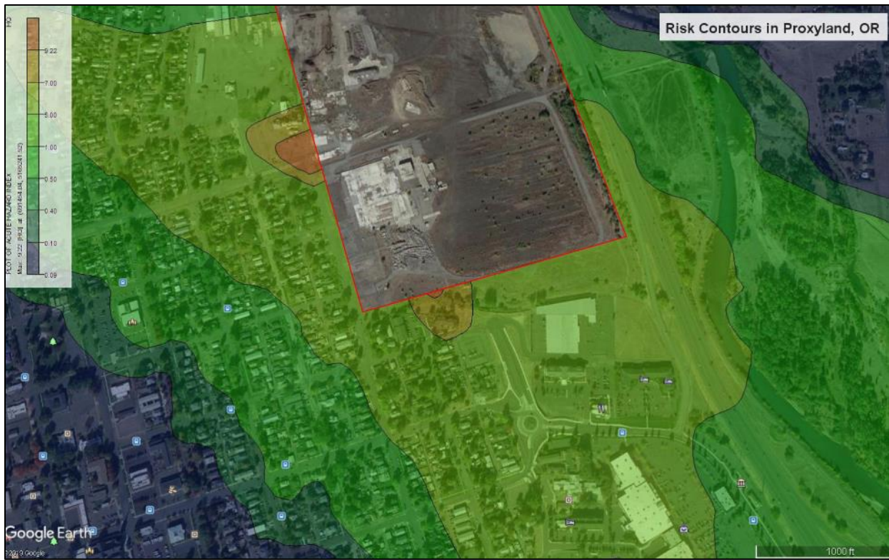
Figure 4. Example of Map From Oregon Showing Off-Site Noncancer Acute Impacts as Hazard Index
