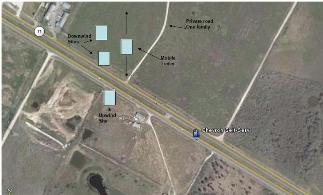
Figure 3. Sampling locations at the Highway 71 sampling site
