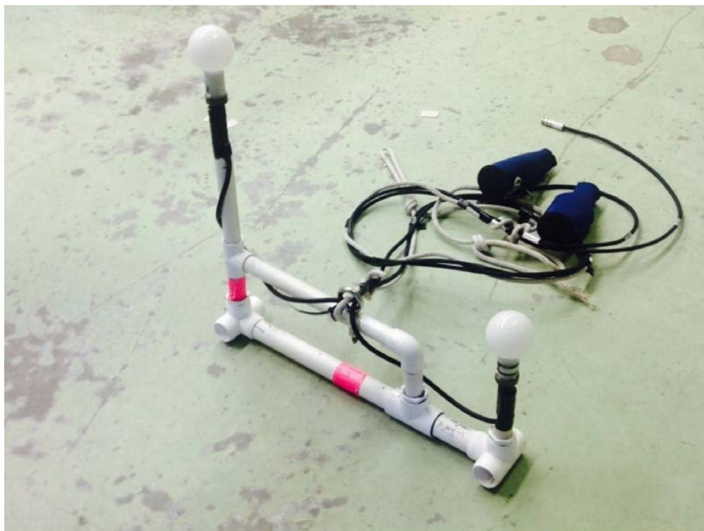
Figure 1. Example of a lowering frame with paired LI-193SA spherical quantum sensors.
