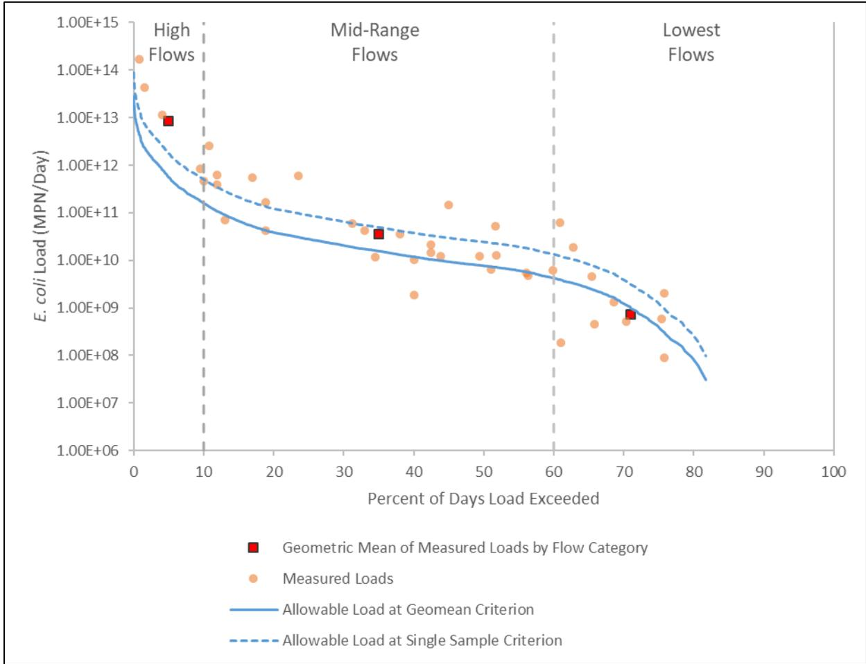
**Figure 11. Load Duration Curve for Arenosa Creek (AU 2453C\_01) at station 13295**
