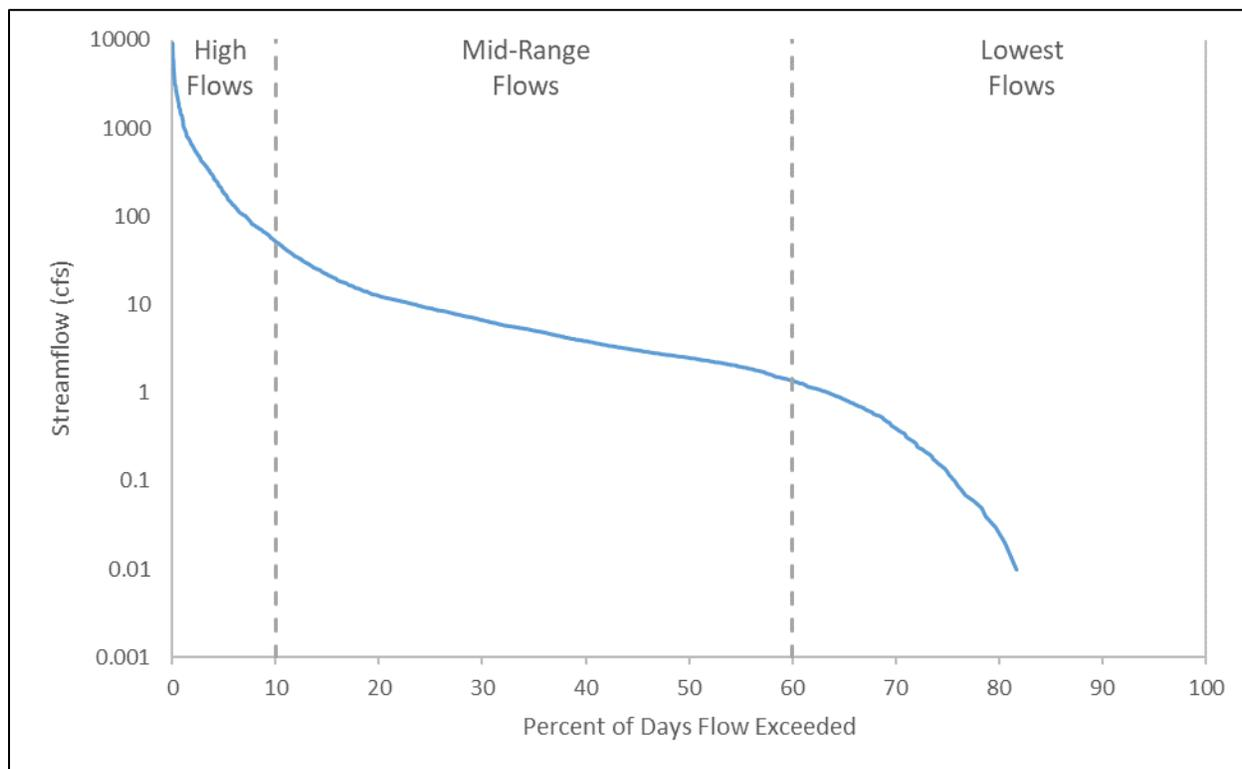
**Figure 10. Flow duration curve for Arenosa Creek (AU 2453C\_01) at station 13295**
