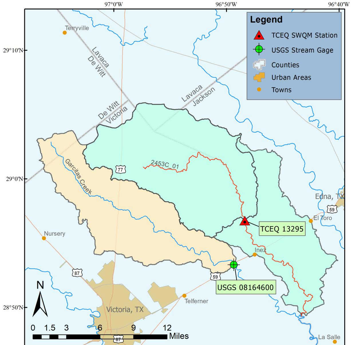
**Figure 9. USGS streamflow gage and watershed used in streamflow development for Arenosa Creek.**
