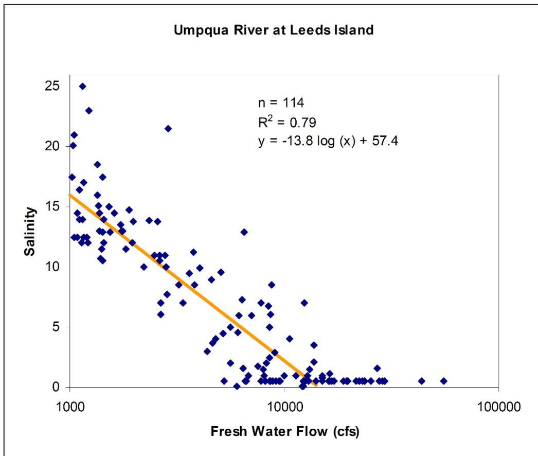
**Figure A-1. Example of salinity to flow regression from Umpqua Basin Tidal streams (ODEQ, 2006).**
