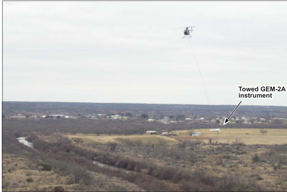
Figure 6. Geophex GEM-2A in flight above the Colorado River near Robert Lee, Texas.
