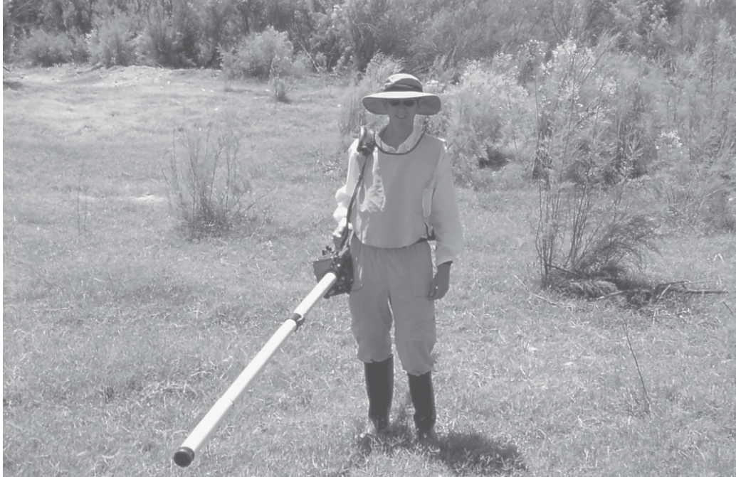
Figure 5. Geonics EM31 ground conductivity meter.
