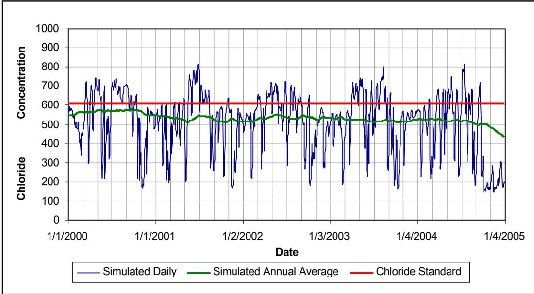
Figure 20: Simulated Chloride Concentrations at Station 12430 under TMDL Allocation
