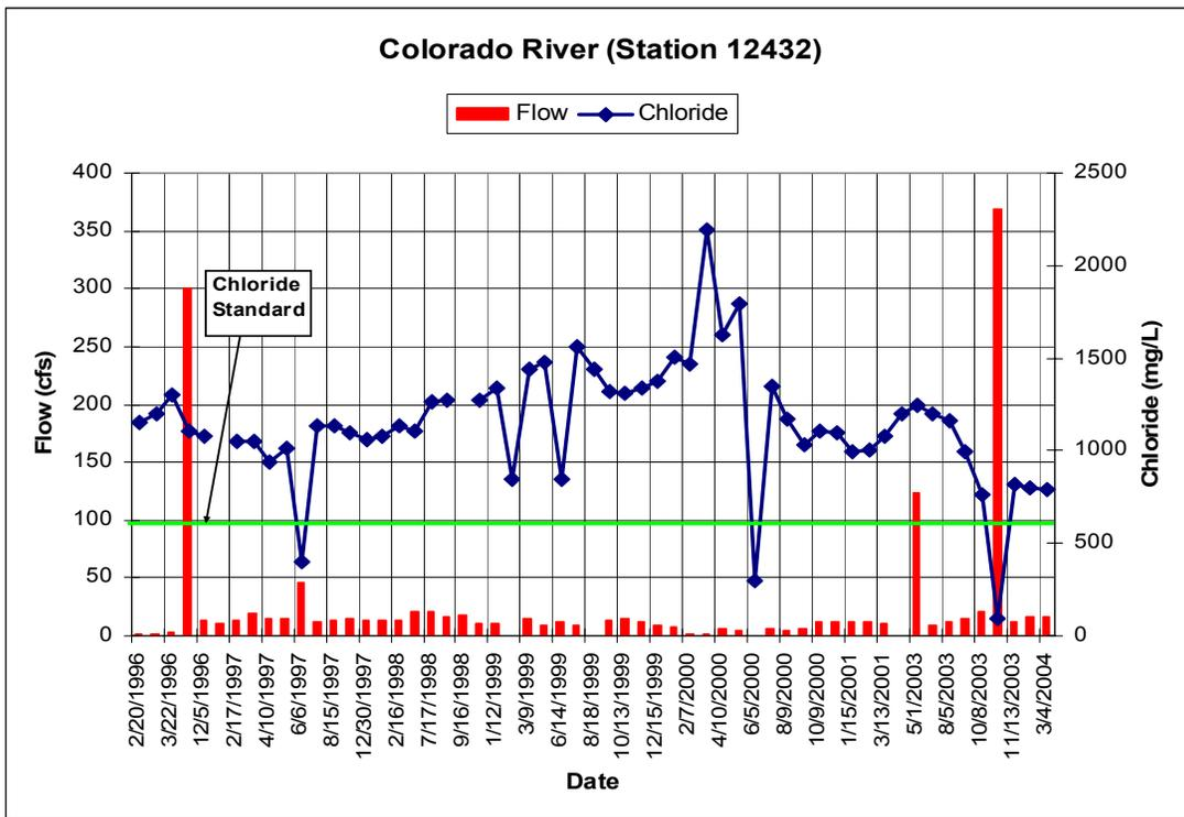
Figure 9: Flow and Chloride Concentrations at Station 12432
