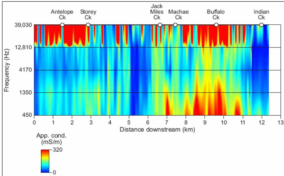
Conductivity using all frequencies acquired during the airborne stream-axis survey. The shallowest-exploring frequency is along the top of the image and the deepest-exploring frequency is along the bottom. (Paine et al, 2005)
