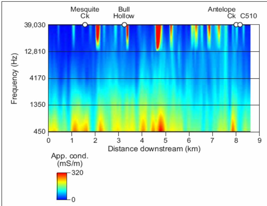
Conductivity using all frequencies acquired during the airborne stream-axis survey. The shallowest-exploring frequency is along the top of the image and the deepest-exploring frequency is along the bottom (Paine et al, 2005)
