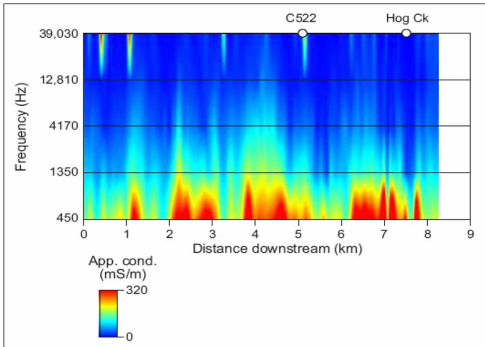
Conductivity using all frequencies acquired during the airborne stream-axis survey. The shallowest-exploring frequency is along the top of the image and the deepest-exploring frequency is along the bottom. (Paine et al, 2005)
