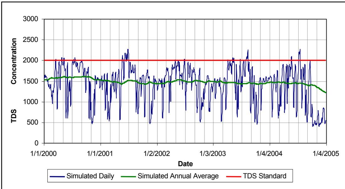
Figure 21: Simulated TDS Concentrations at Station 12430 under TMDL Allocation
